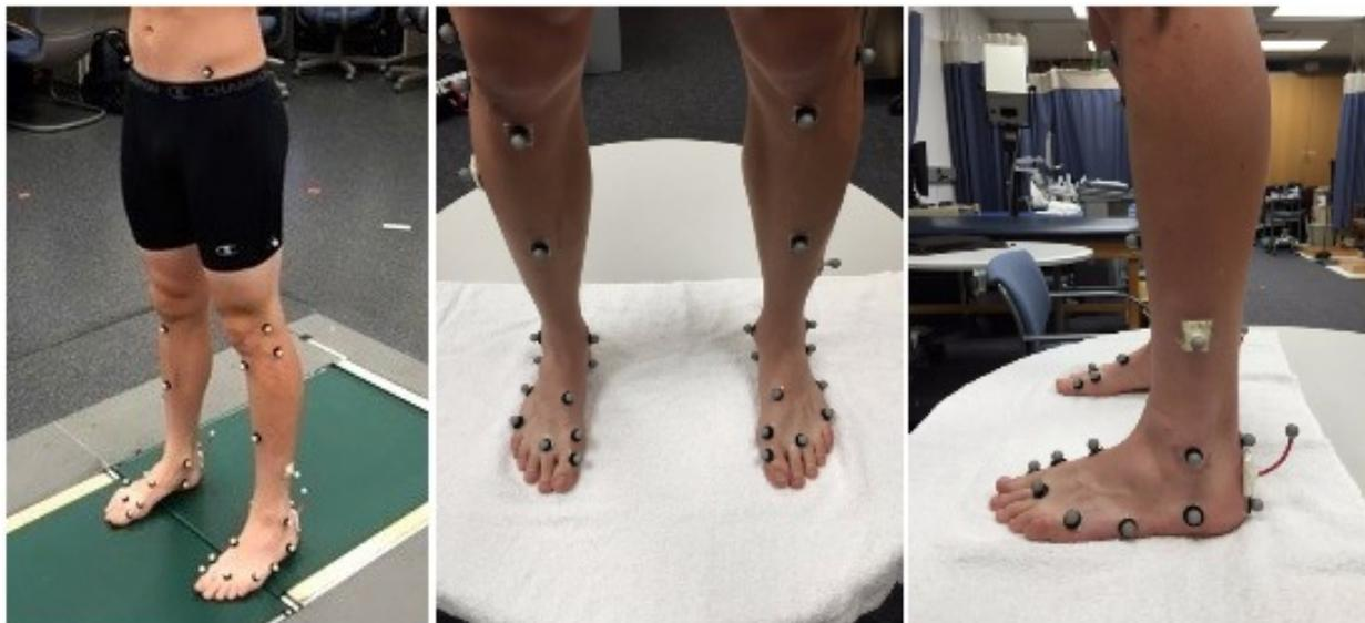
Figure 2. Vicon Oxford Foot Model marker placement
