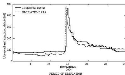
**Figure 5.** Observed and simulated hourly flows for the flood event in Upper Iskar River in November, 2004 [Ribarova et al., 2008a]
