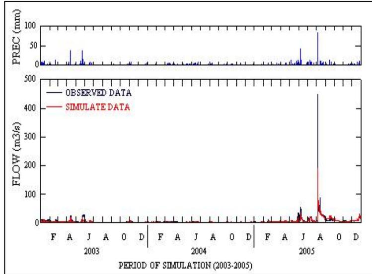
**Figure 3.** Observed and simulated daily flows and precipitation at Dolni Bogrov Gauge Station – Lesnovska River
