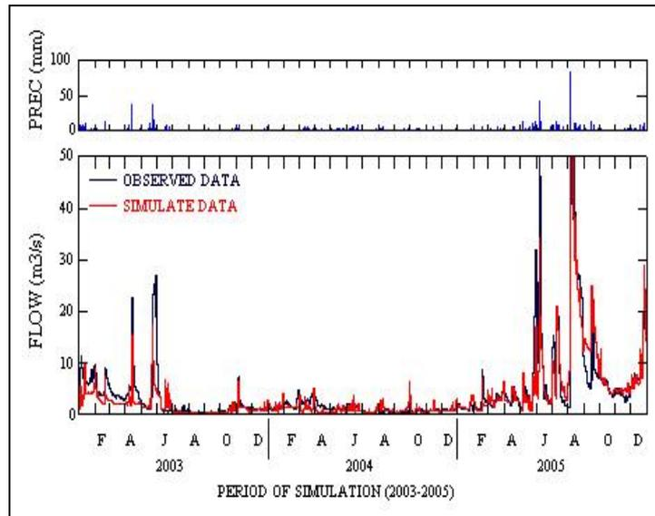
**Figure 4.** Low-range (less than 50 m<sup>3</sup>/s): observed and simulated daily flows and precipitation at Dolni Bogrov Gauge Station – Lesnovska River
