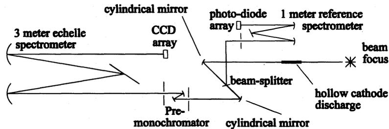
FIG. 1.—Schematic diagram of the high-sensitivity absorption experiment
