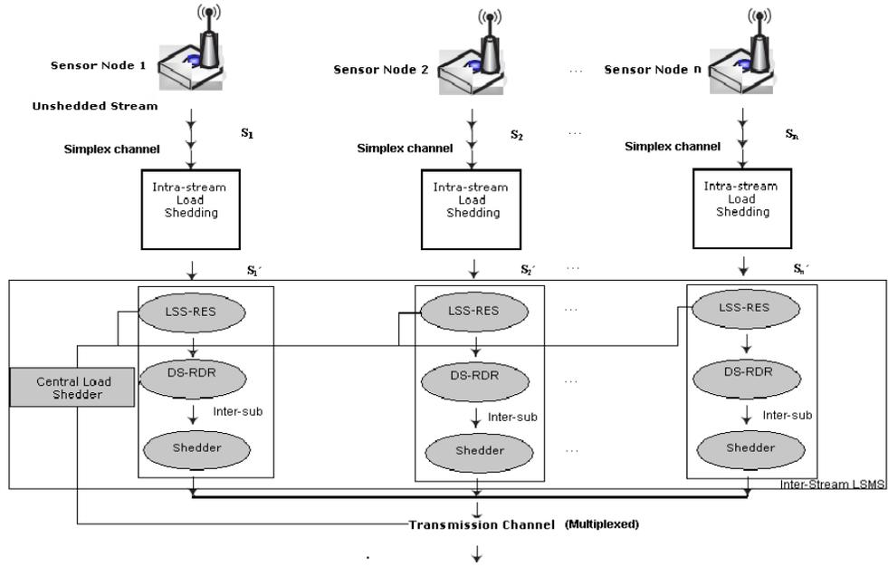
Figure 3.9: Load shedding sub-system architecture in our DSMS
