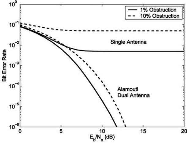
Fig. 5. BER versus  $E_b/N_0$  for an air vehicle engaged in a roll for single antenna and Alamouti dual antenna transmission with QPSK symbols evaluated using the closed-form BER solution. Signal from each antenna is obstructed 1% or 10% of the time during the maneuver.
