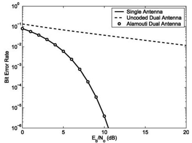
Fig. 4. BER versus  $E_b/N_0$  for an air vehicle engaged in a roll for single antenna, uncoded dual antenna, and Alamouti dual antenna transmission with QPSK symbols evaluated using the closed-form BER solution. Antenna obstruction is neglected.
