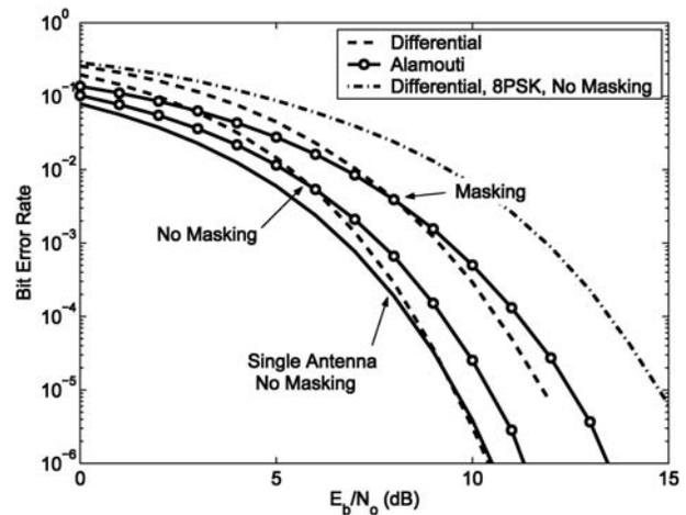
Fig. 10. Comparison of BER versus  $E_b/N_0$  for differential and Alamouti codes using the full system simulation used for Fig. 9 with and without masking included. Results for differential codes using 8PSK symbols (no masking included) are also shown.
