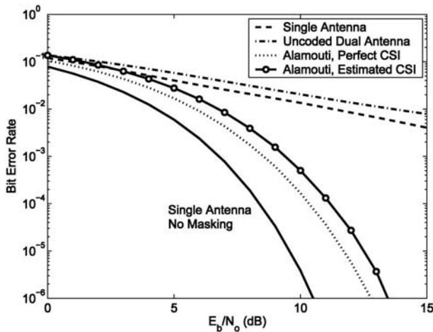
Fig. 9. BER versus  $E_b/N_0$  obtained from a full system simulation for an aircraft engaged in a roll when channel estimation ( $N_T = 8$ , 5% of symbols devoted to training) and masking are included for various signaling schemes.
