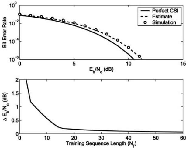
Fig. 6. Top Plot: BER versus  $E_b/N_0$  for a training sequence of length  $N_T = 8$  obtained from the approximate statistical analysis (“Estimate”) and detailed system simulations. Result for perfect CSI is shown for comparison. Bottom Plot: Required increase in signal strength  $\Delta E_b/N_0$  to achieve a BER of  $10^{-5}$  relative to the case where perfect CSI is available as a function of  $N_T$ .
