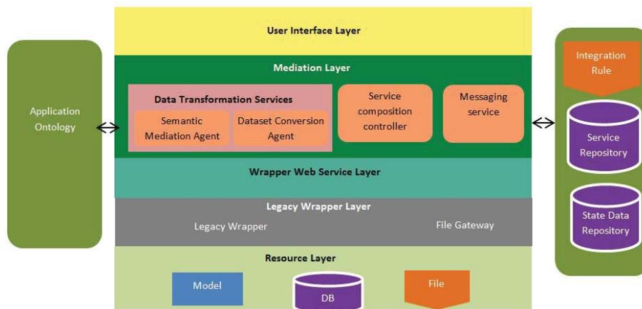
Figure 1: Conceptual architecture of the model integration framework
