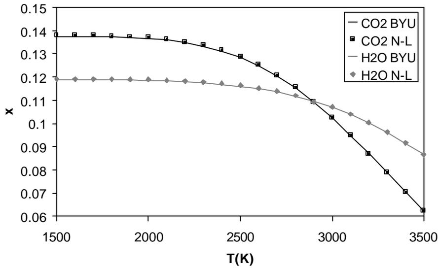
Figure 6.4. Temperature vs. CO<sub>2</sub> and H<sub>2</sub>O Mole Fractions
