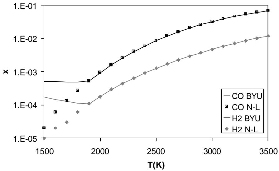
Figure 6.5. Temperature vs. CO and H<sub>2</sub> Mole Fractions
