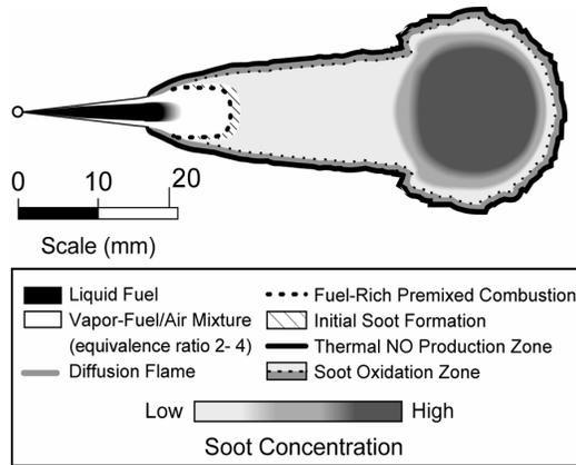
**Figure 2.1. Quasi-steady diesel combustion plume as presented by Dec (1997) [2].
