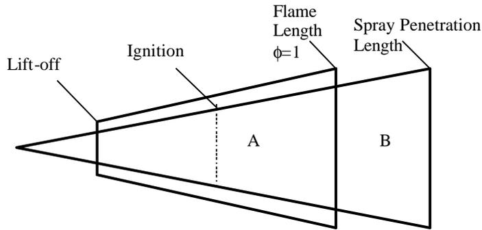
**Figure 4.1. Spray Geometry used for Heat Release Calculations.**
