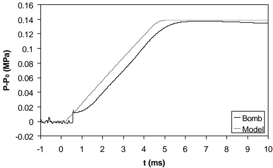
**Figure 6.22. Sandia Bomb Pressure Rise Using the 100- $\mu$ m Nozzle with Extra Heat Transfer.**
