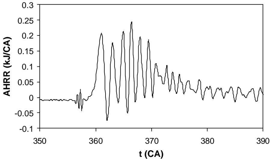
**Figure 6.13. Apparent Heat Release from Unfiltered Pressure Data**
