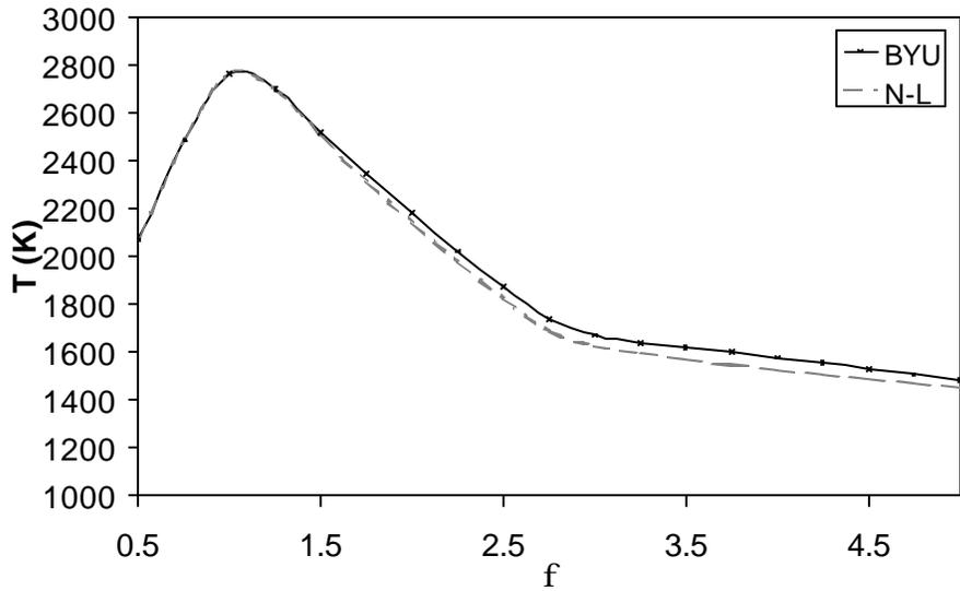
**Figure 6.10. Adiabatic Flame Temperature vs. Equivalence Ratio**
