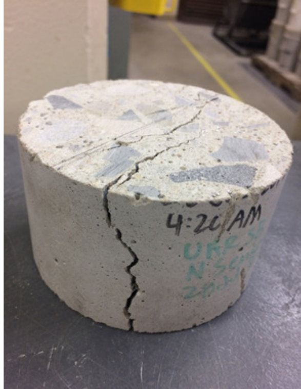
Figure D-9: Typical Upper Ridge Road SB TSMR specimen after splitting tensile strength testing.
