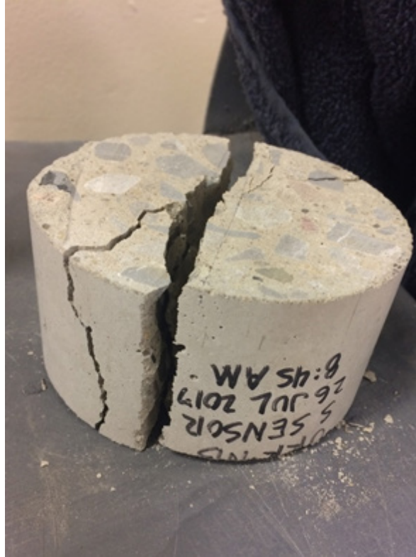
Figure D-11: Typical Upper Ridge Road NB conventional concrete specimen after splitting tensile strength testing.
