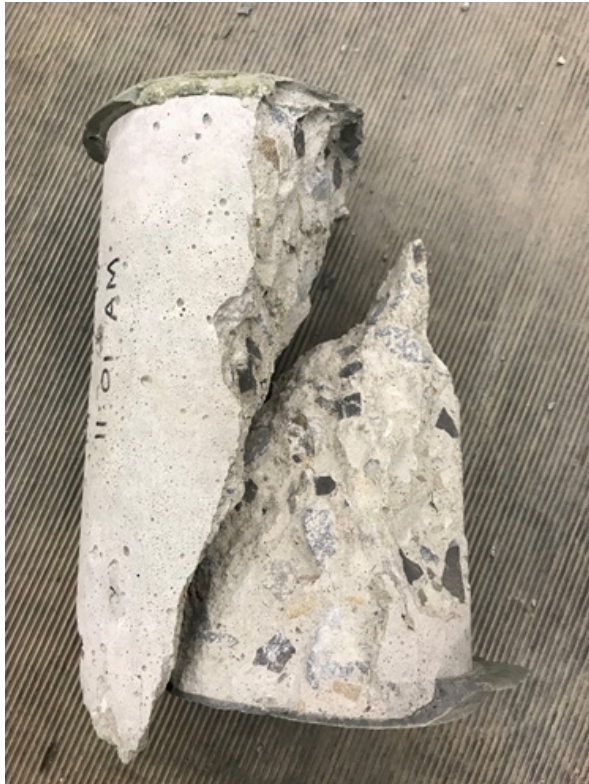
Figure D-4: Typical Wolverine Way SB conventional concrete specimen after compressive strength testing.
