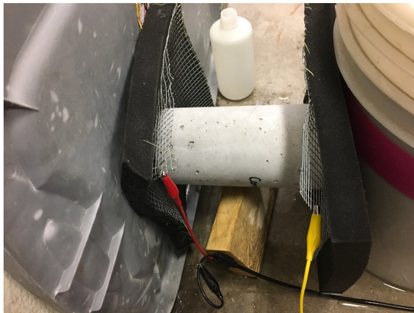
Figure 3-8: Electrical impedance testing of a cylindrical specimen.
