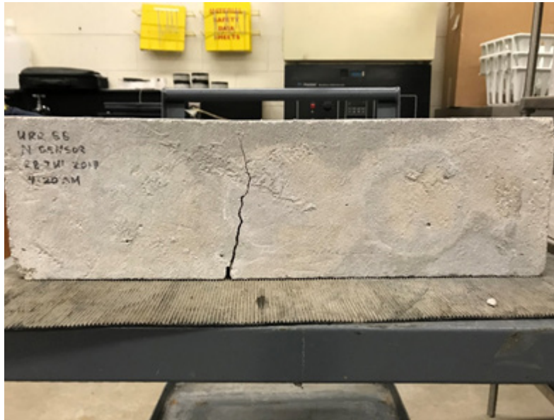
Figure D-5: Typical Upper Ridge Road SB TSMR specimen after flexural strength testing.
