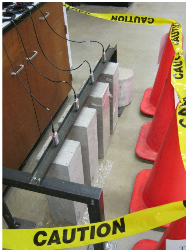
Figure 3-7: Shrinkage testing of beam specimens.
