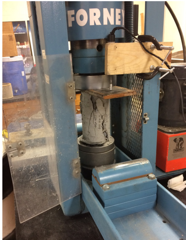
Figure 3-9: Compressive strength testing.
