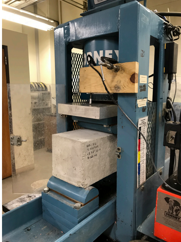
Figure 3-10: Flexural strength testing.
