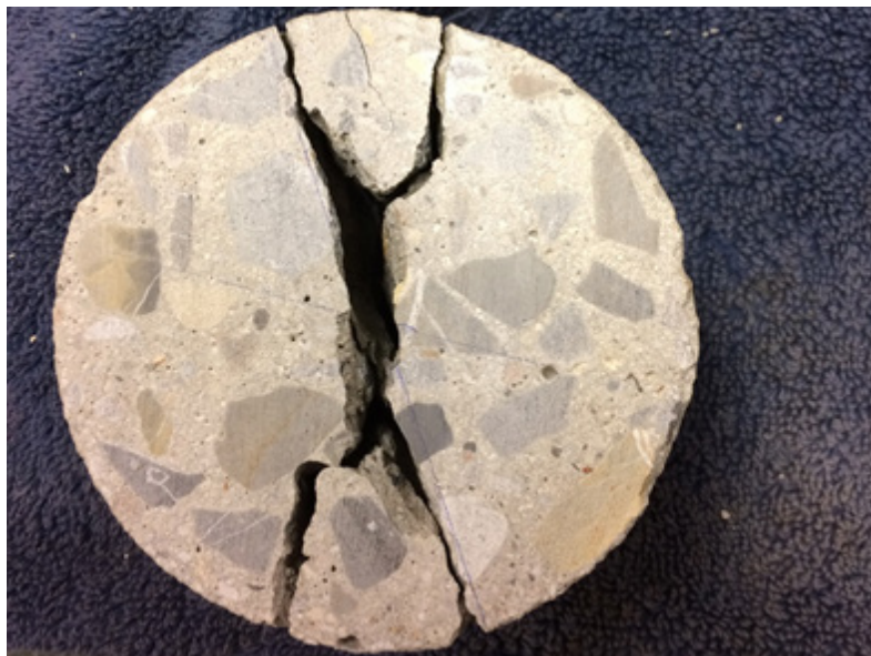
Figure D-12: Typical Wolverine Way SB conventional concrete specimen after splitting tensile strength testing.
