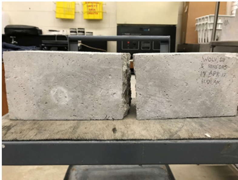
Figure D-8: Typical Wolverine Way SB conventional concrete specimen after flexural strength testing.
