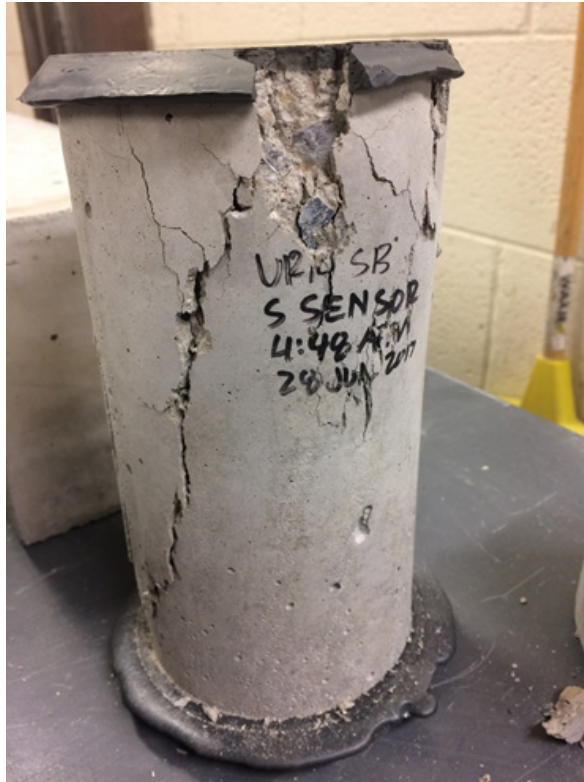
Figure D-1: Typical Upper Ridge Road SB TSMR specimen after compressive strength testing.
