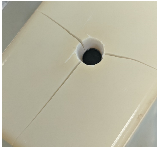
Figure 4-5: Digital ABS Benchmark Mold Cracking Just Prior to Failure
