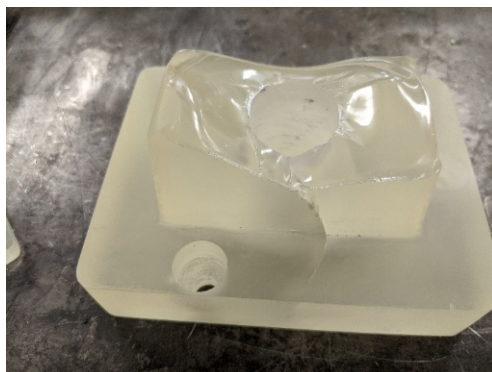
Figure 4-12: High Temp Resin A-Side Insert Failure
