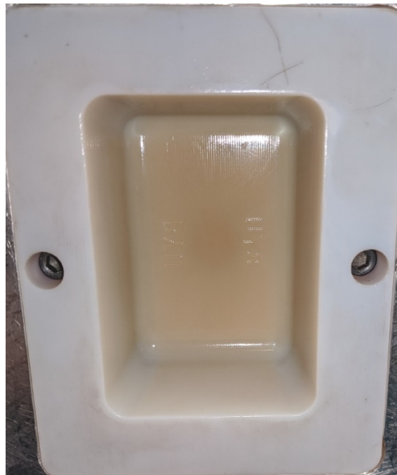
Figure 4-8: Digital ABS Benchmark Mold B-Side After Failure
