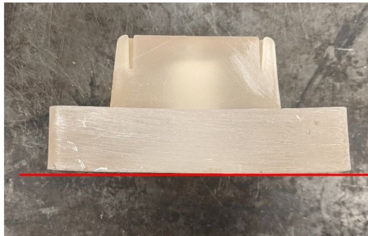
Figure 3-13: High Temp Resin A-Side Curing Damage
