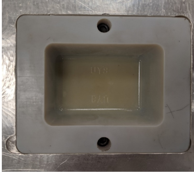
Figure 3-12: Digital ABS B-Side Mold Prepped for Testing
