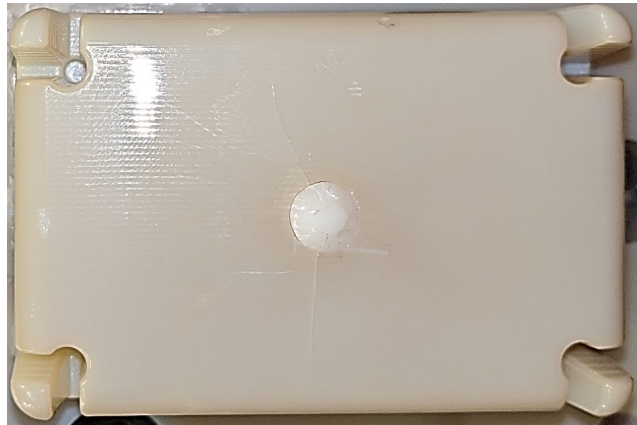
Figure 4-4: Digital ABS Benchmark Mold Initial Cracking
