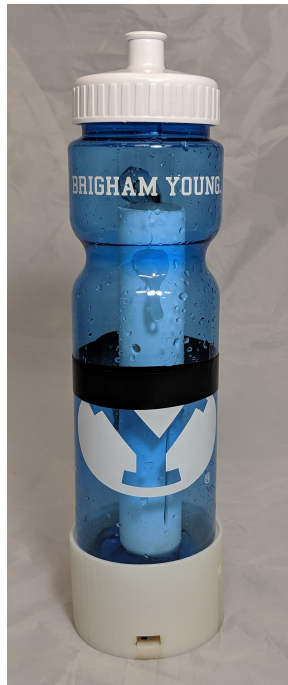
Figure 6.4: Our instrumented water bottle. The bottle tracks a hiker's water intake and displays a color via an RGB LED which indicates the hiker's estimated hydration level.
