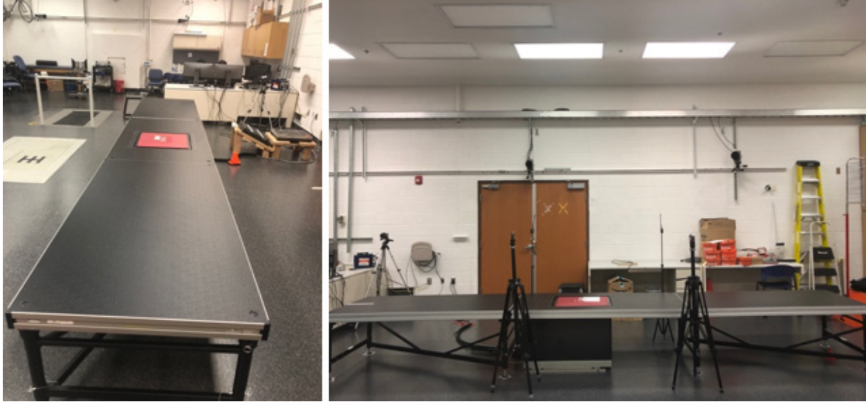
Figure 3. Walkway with FootSTEPS and laser timers (L = front view of walkway with FootSTEPS in middle; R = side view of walkway including laser timers).
