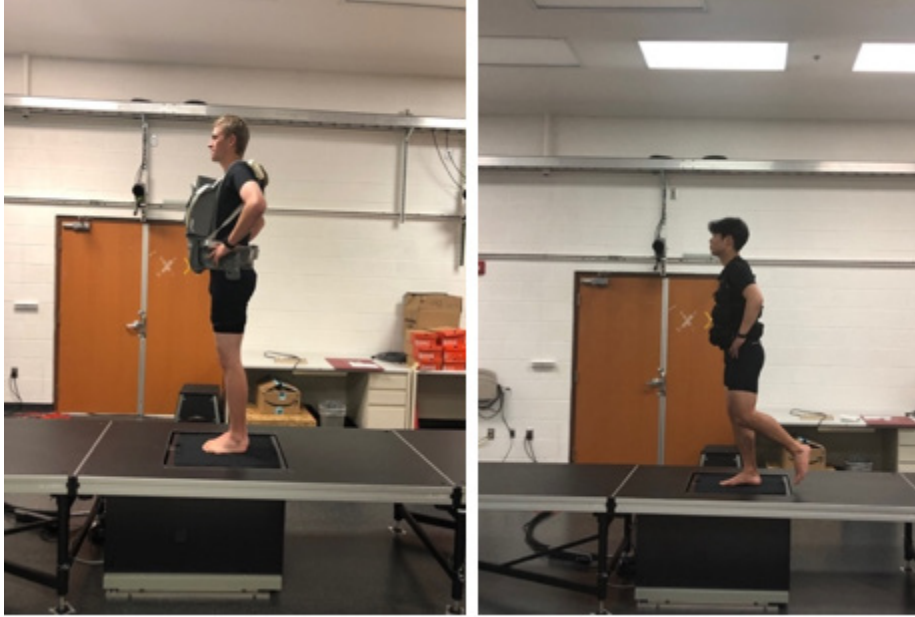
Figure 2. Standing Trials (L = both feet in FV; R = single foot in EV)
