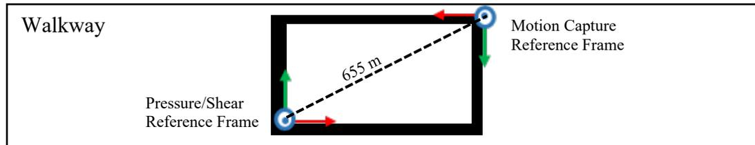
**Figure 2.** Spatial alignment. The walkway (outer white rectangle) with the FootSTEPS device (black rectangle) and pressure/shear measurement film (inner white rectangle). The pressure/shear reference frame is located at the lower left corner of the film while the motion capture reference frame is located at the upper right corner of the device. The offset measured between reference frame origins is provided (1.02 m longitudinally and 1.16 m laterally).
