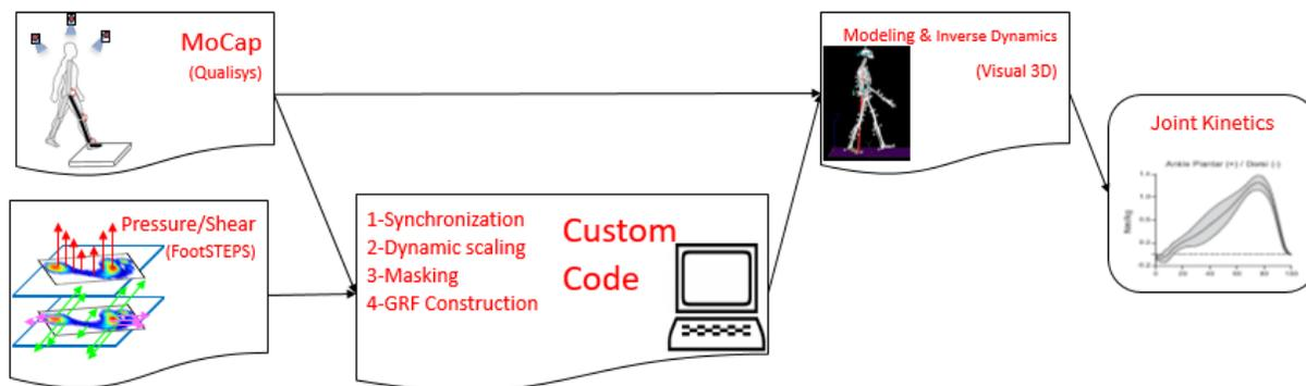
**Figure 3.** Visual workflow of system integration. Motion capture and pressure/shear data were collected simultaneously and imported into custom software. Four main integration steps were accomplished and final segment GRFs were exported. GRFs and motion capture were then imported into Visual 3D software for modeling and inverse dynamics, resulting in foot joint kinetics.
