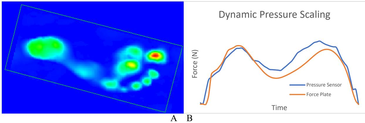
**Figure 4.** Dynamic pressure scaling. Representative composite pressure image and an extracted foot region (A). The region of interest was defined from motion capture markers superimposed onto the composite image. The total vertical force from this region is shown along with the vertical force plate signal from the same trial (B), prior to dynamic scaling.
