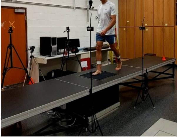
**Figure 1.** Participant on walkway. A 5.5 m long walkway was modified by cutting a hole in the center so that the pressure/shear sensor was flush with the walking surface. The timing lights for speed measurements are also visible.
