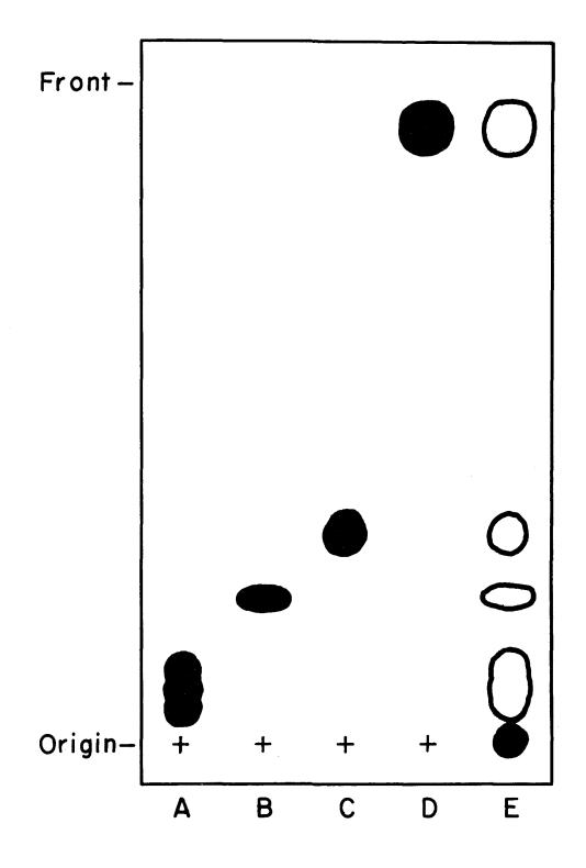
Fig. 3. Thin-layer chromatography of phospholipids on a silica gel G layer. Solvent: chloroform-methanol-acetic acidwater, 50:25:8:4. Key: A, phosphatidyl choline; B, Phosphatidyl serine; C, phosphatidyl ethanolamine; D, mixture of diolein, triolein, oleic acid, cholesterol and cholesterol oleate; E, lipids from the quasi-crystalline material. Visualization was with 5% sodium dichromate in 50% sulfuric acid at 200° for 30 min.
