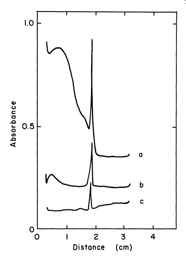
Fig. 15. Polyacrylamide gel electrofocusing of quasi-crystalline material. Key: a, scan of the gel at wavelength of 280 nm;
