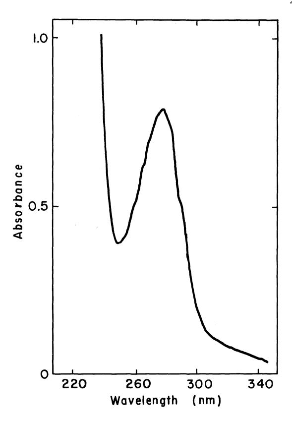
Fig. 6. Absorption spectrum of lipid from a chloroethanol extraction of the quasi-crystalline material. The solvent was 2-chloroethanol adjusted to pH 8 with ammonium hydroxide.
