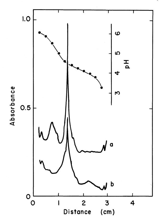
Fig. 16. Polyacrylamide gel electrofocusing of hydrolyzed quasicrystalline material. Key: a, scan of the gel at a wavelength of 280 nm; b, scan of the gel at a wavelength of 260 nm. Samples were transferred to 6 M guanidine hydrochloride after hydrolysis. The gels were scanned immediately after electrofocusing and were not stained or fixed.
