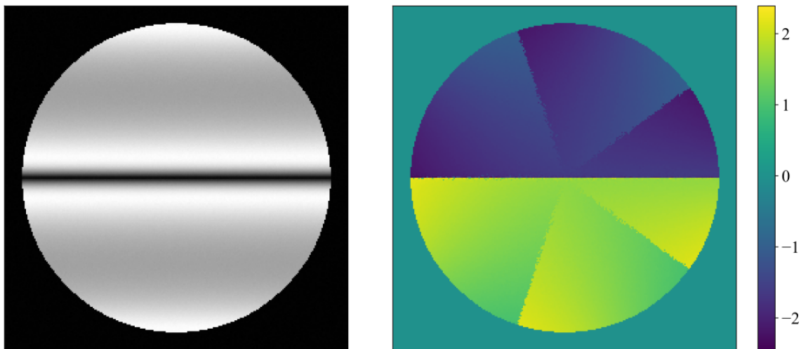
Figure 4.5: The left image shows the SOS coil combined 0^\circ phase cycle (SNR=47). The right image shows the simple phase substitution for the SOS reconstruction with the phase discontinuities predicted in the Theory section. The discontinuities lie along the coil intersections as well as along the horizontal bSSFP “null.”
