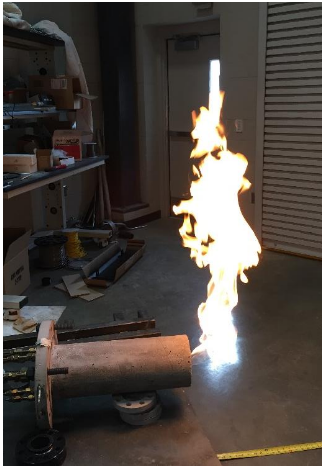
Figure 4-6: Preliminary Burner Testing at 50 \text{KW}_{\text{th}} .
