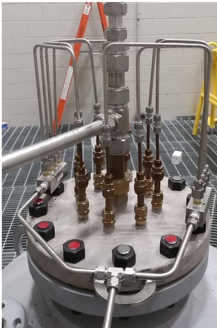
Figure 4-8: Photograph of Tubing, Swagelok Connections, and Manifold Connecting to the Burner.
