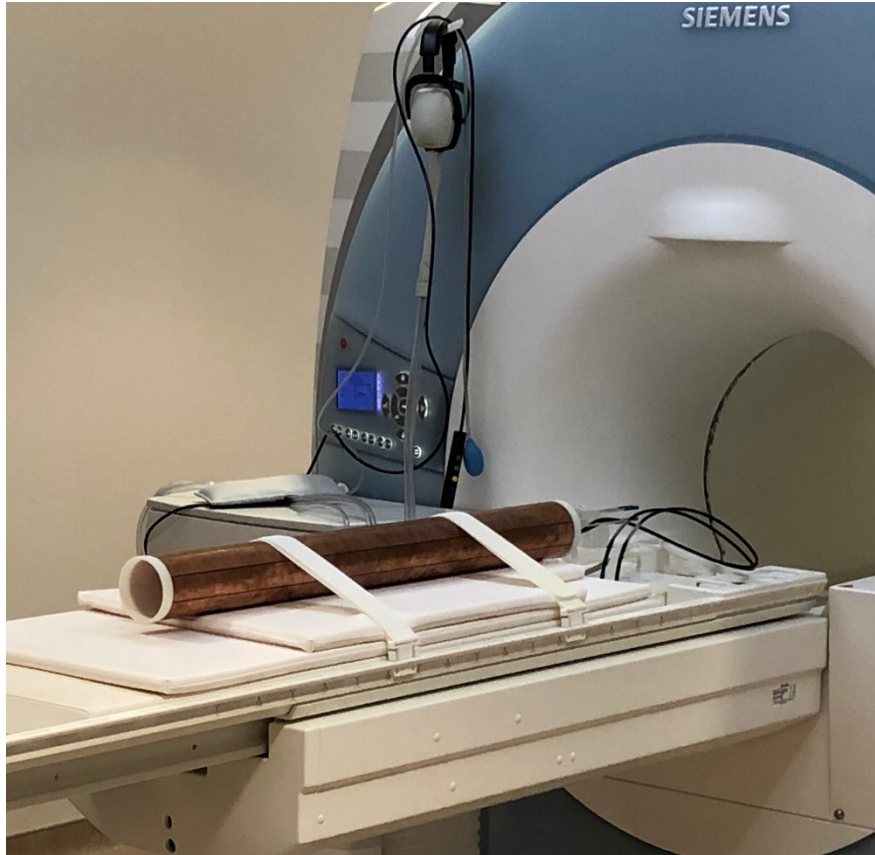
Figure 3.1: MRI Scanning Protocol Setup. The mouse coil was strapped to the table and elevated to be directly in iso-center, which was required by the UTE scans. The anesthetic delivery system was sent through the bore of the magnet.
