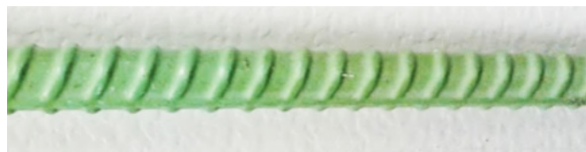
Figure 3-6: Photo of Steel-Epoxy Coated Rebar Configuration
