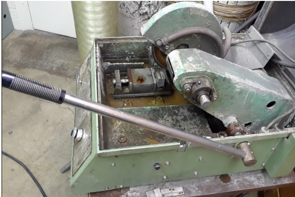
Figure 3-11: Cut-off Saw Jig with Diamond Coated Blade Specimen Polishing
