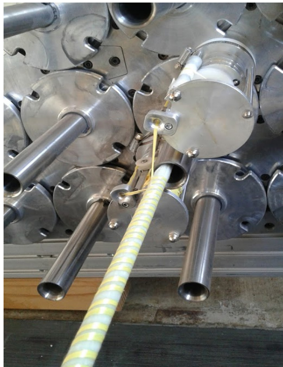
Figure 7-5: Fiberglass/Epoxy Rebar Comprising Prepreg Tows Being Consolidated by Bobbins on Braiding Wall
