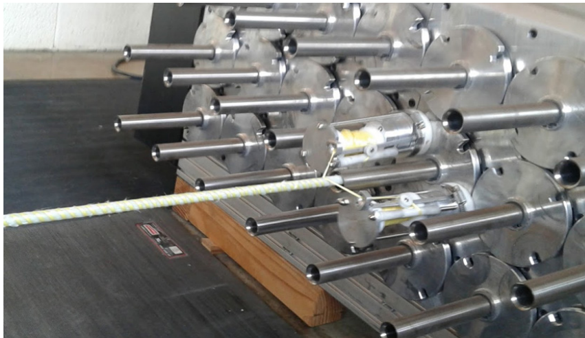
Figure 3-2: Two Bobbins Braiding a Sleeve on the Core for Consolidation
