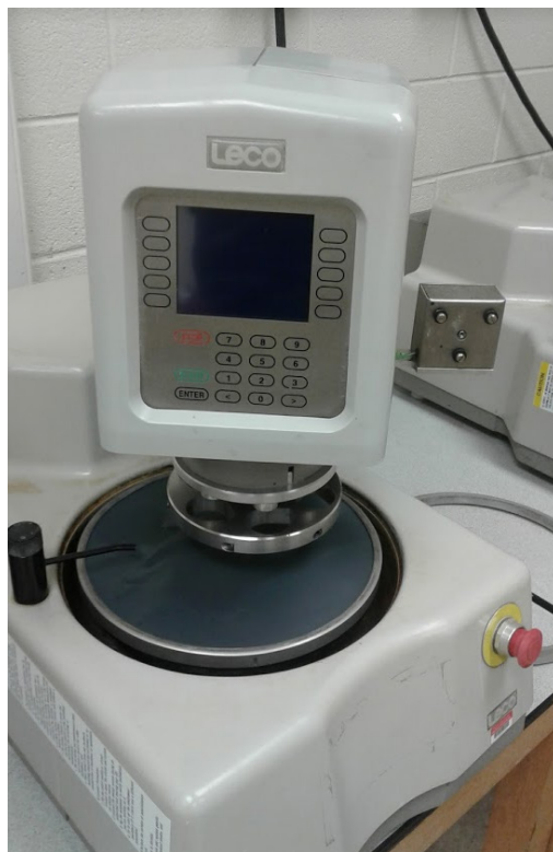
Figure 3-12: Photograph of Leco CM-10 Polishing Machine
