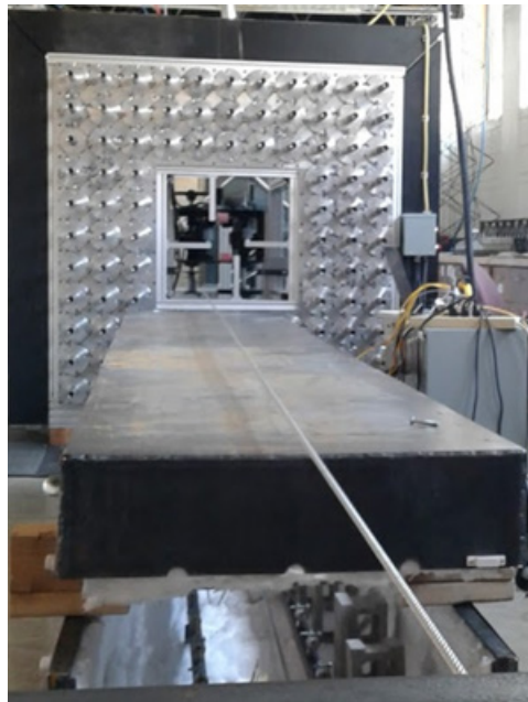
Figure 3-8: Rebar Manufacturing on Prototype IsoTruss Machine with Inline Oven
