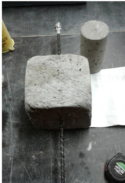
Figure 2-3: Rebar Embedded in Concrete
