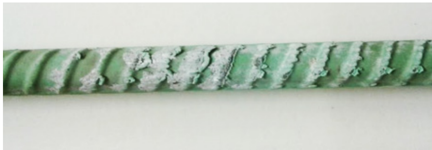
Figure 4-41: Concrete Shear Failure on Steel Epoxy Coated Rebar
