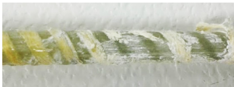
Figure 4-36: Rebar Surface Failure on Manufactured Non-Sand-coated Specimens
