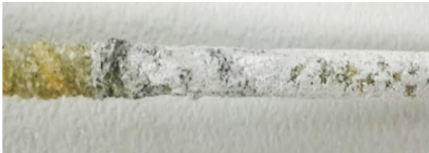
Figure 4-42: Concrete Shear Failure on Manufactured Sand-coated Rebar
