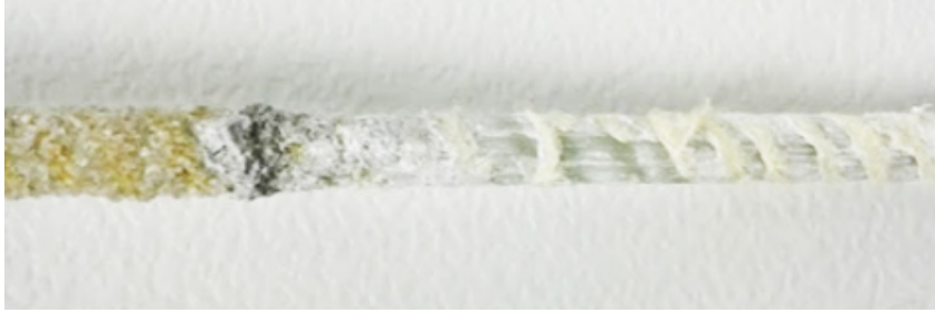
Figure 4-37 Rebar Surface Failure on Manufactured Sand-coated Specimens
