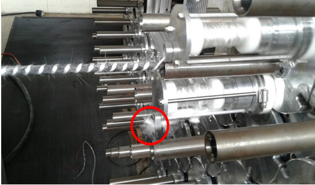
Figure 2-2: Fraying of Fiberglass at the Pay-Out Eye during Manufacturing of Carbon/Epoxy Core
