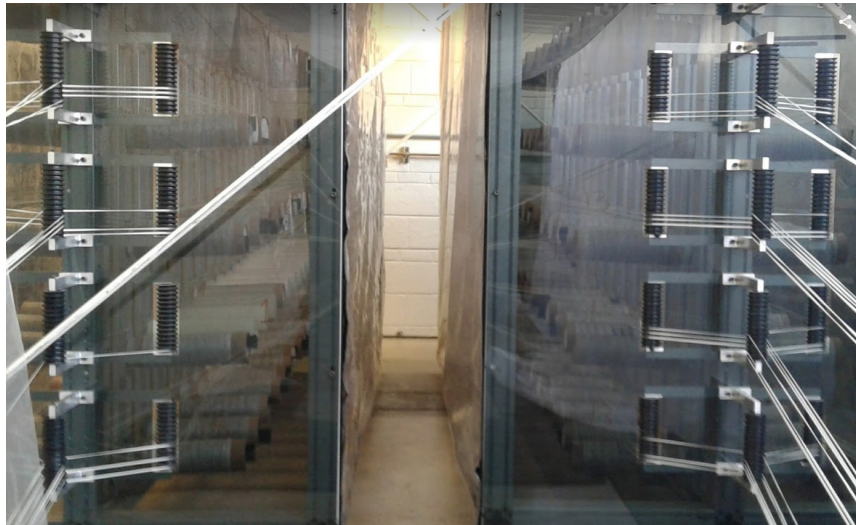
Figure 7-2 Prepreg Tows Being Pulled From the Creel
