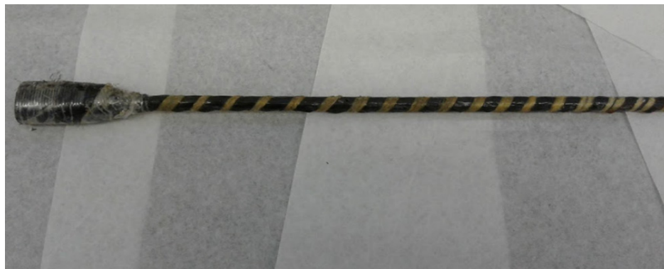
Figure 2-1: Carbon/Epoxy Rebar with Doubler on End for Gripping in Testing Machine
