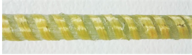
Figure 3-3: Photo of Non-Sand-coated Rebar Configurations
