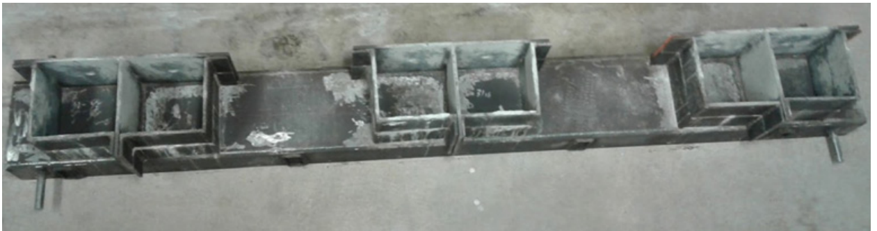
Figure 3-13: Metallic Forms/Casting Fixture
