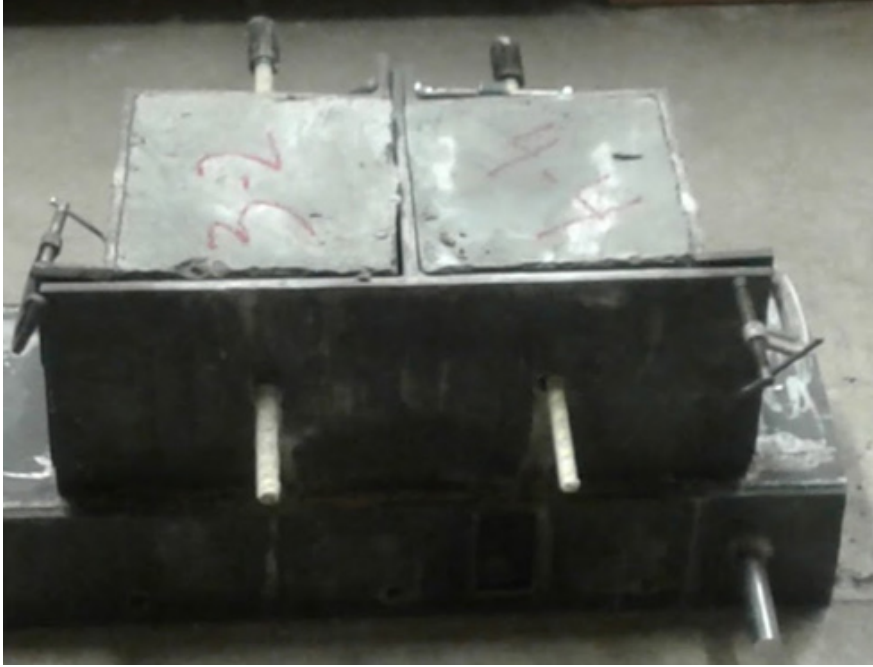
Figure 3-15: Concrete Specimens Cast into Forms and Ready for Stripping
