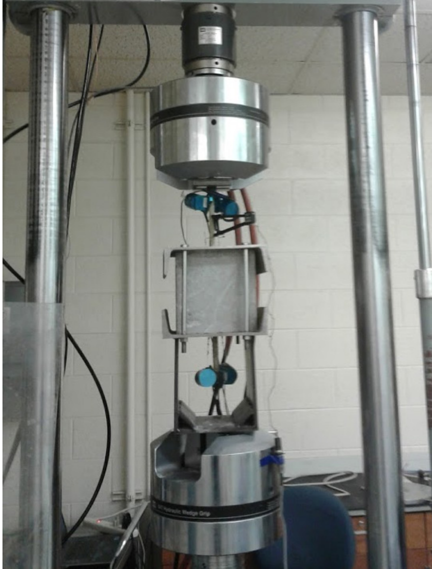
Figure 3-22: Photograph of Test Set-up for Rebar Pull-Out Testing
