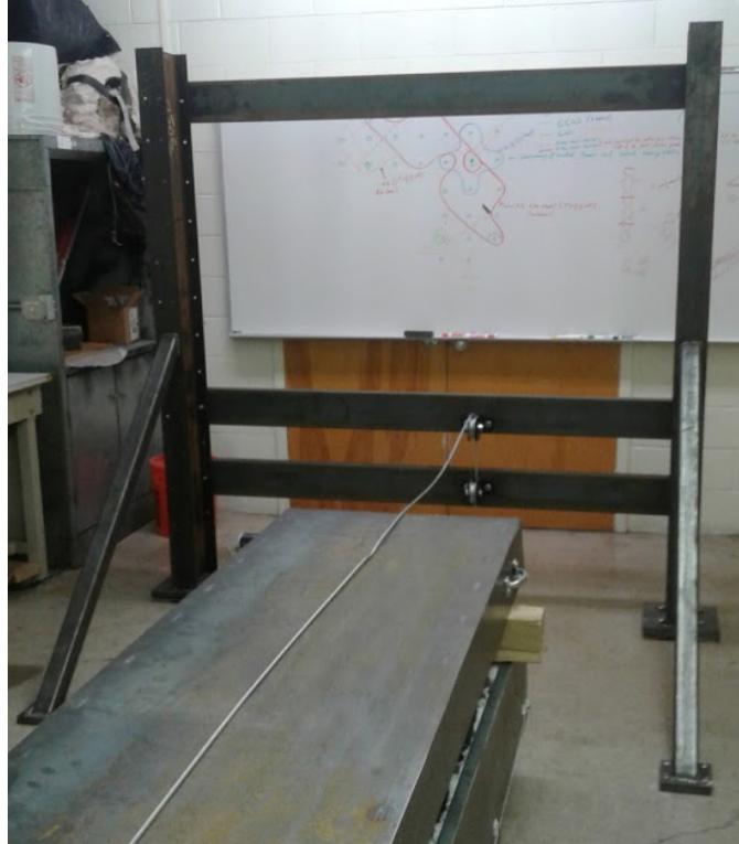
Figure 7-7: Inline Oven and Pulley Frame System for Pulling Small Numbers of Rebar
