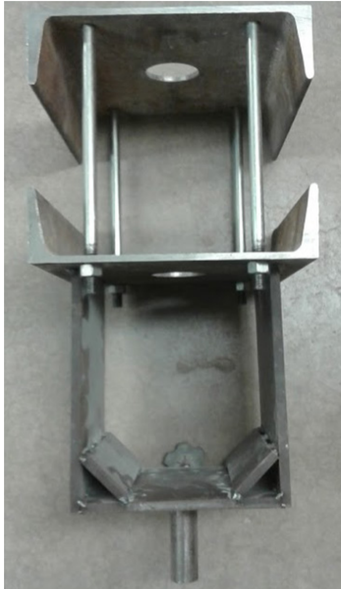
Figure 3-21: Photograph of Testing Fixture for Rebar Pull-Out Testing
