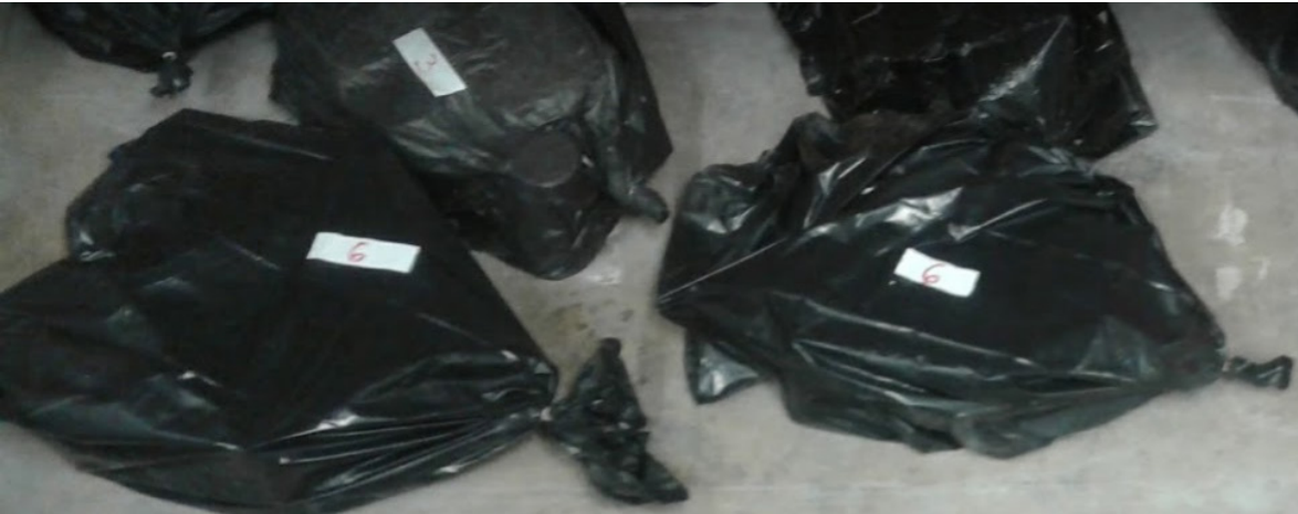
Figure 3-16: Curing of Concrete Specimens in Plastic Bags
