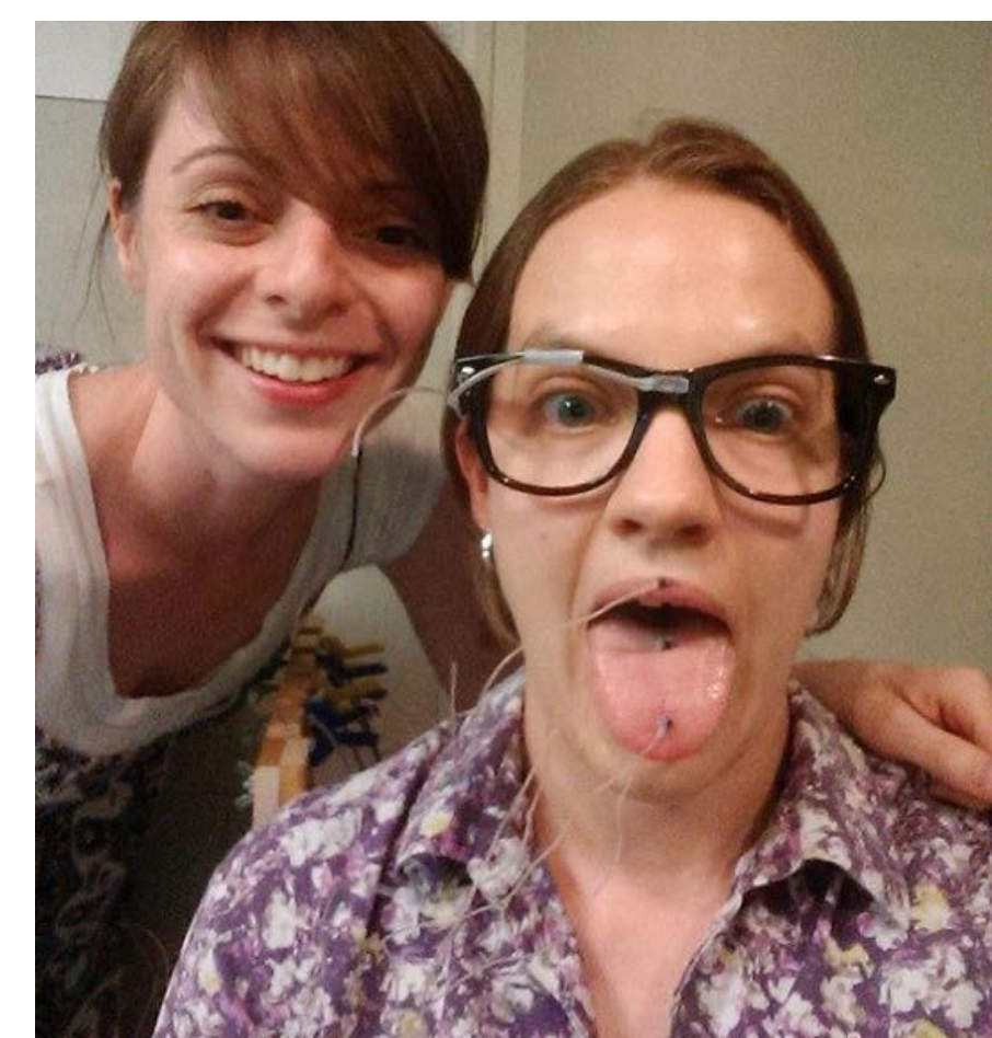
Figure 1. Kinematic recordings were made using the NDI wave system. The picture shows an example the locations of the sensor coils. This investigation examined movement records for the tongue-front marker, located near the tongue tip, and the tongue-middle marker, located near the dorsum of the tongue.
