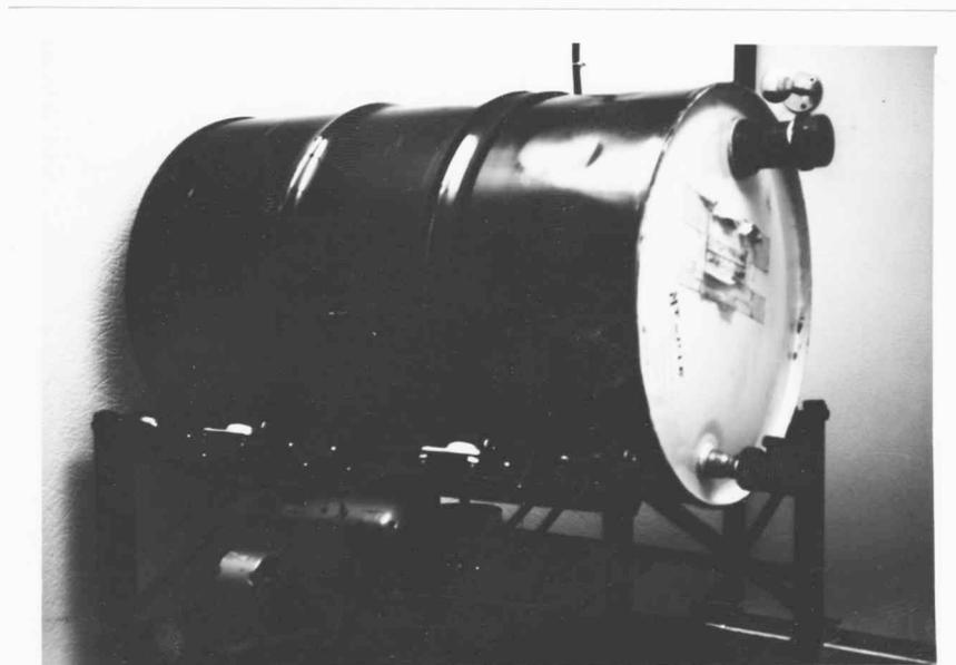
Fig. 20. Drum rotator for masterbatch
