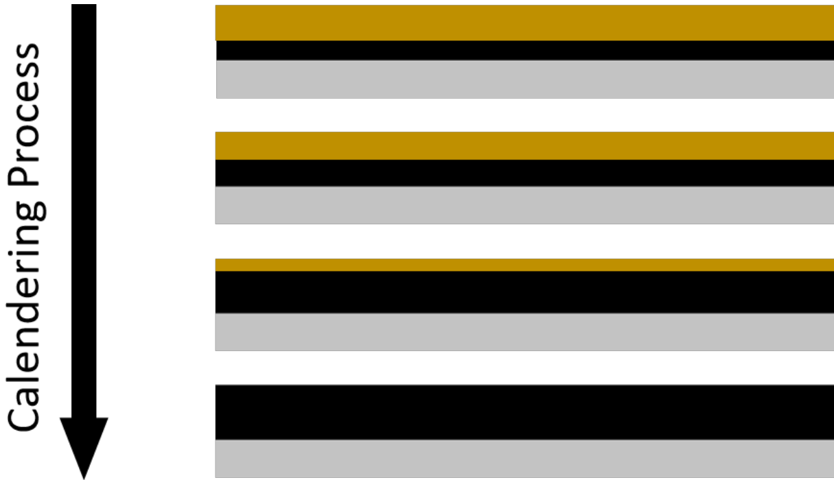
Figure 5.7: A diagram to show the effective thickness change during the first few calendaring processes. The brown layer, black layer and gray layer represent the mass loading layer, effective coating layer and current collector layer, respectively
