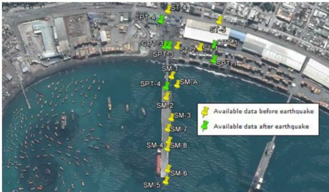
Figure 6-5: Locations of Boreholes and Geotechnical Soundings near the North Pier (Ledezma & Tiznado, 2017)
