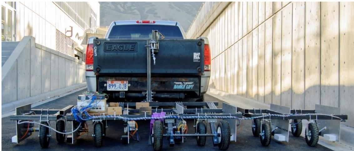
Figure 3-4. Unfolded 3.76 m trailer ready for scanning a bridge lane.
