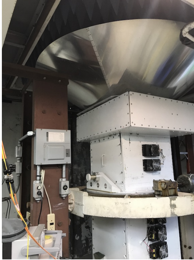
Figure 4.5: Front-end receiver system and array mounted in the OTF.
