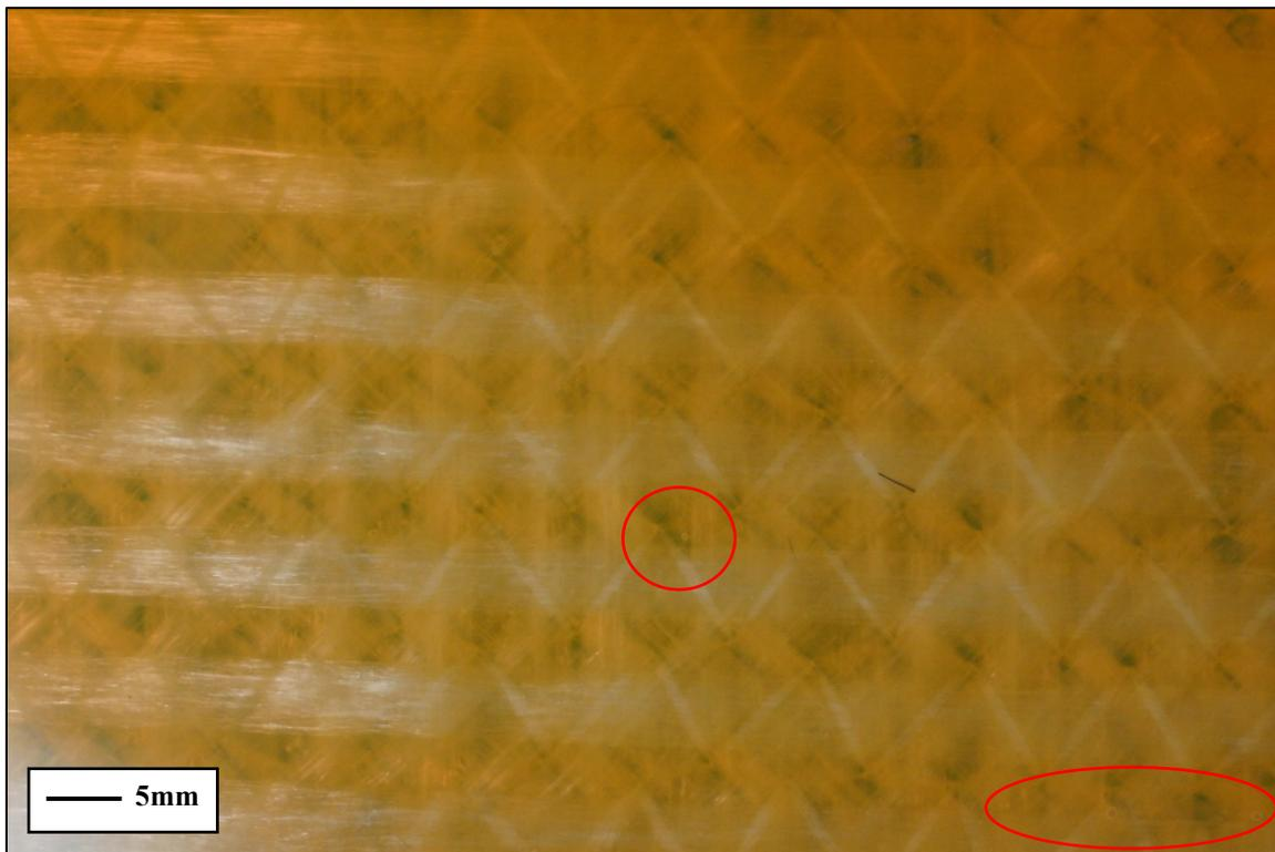
**Figure 4-3 - Fiberglass with Oil/UV Dye Mix in Room Lighting**
