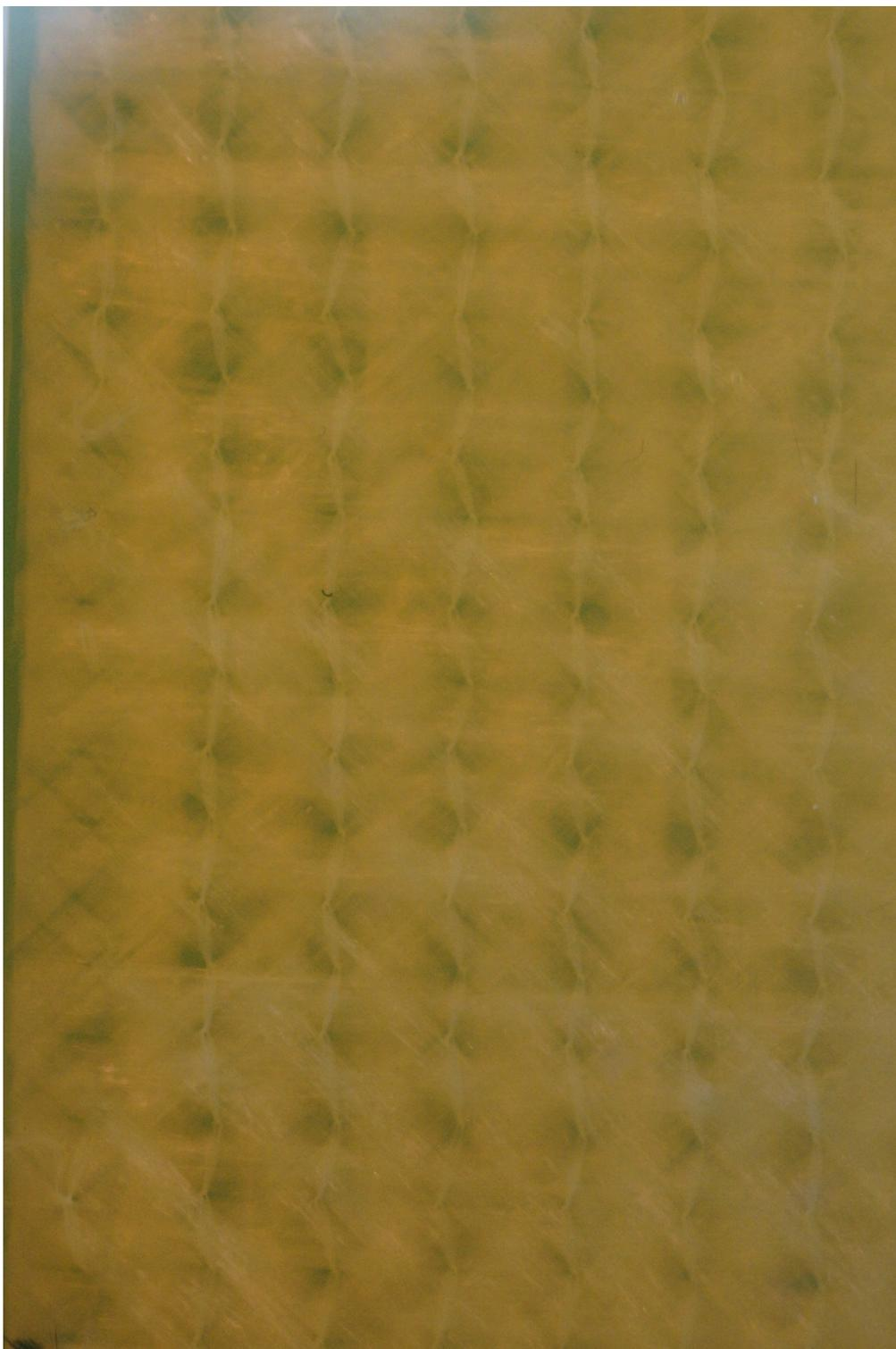
**Fiberglass with Test Fluid/UV Dye Mix and UV Lighting**
