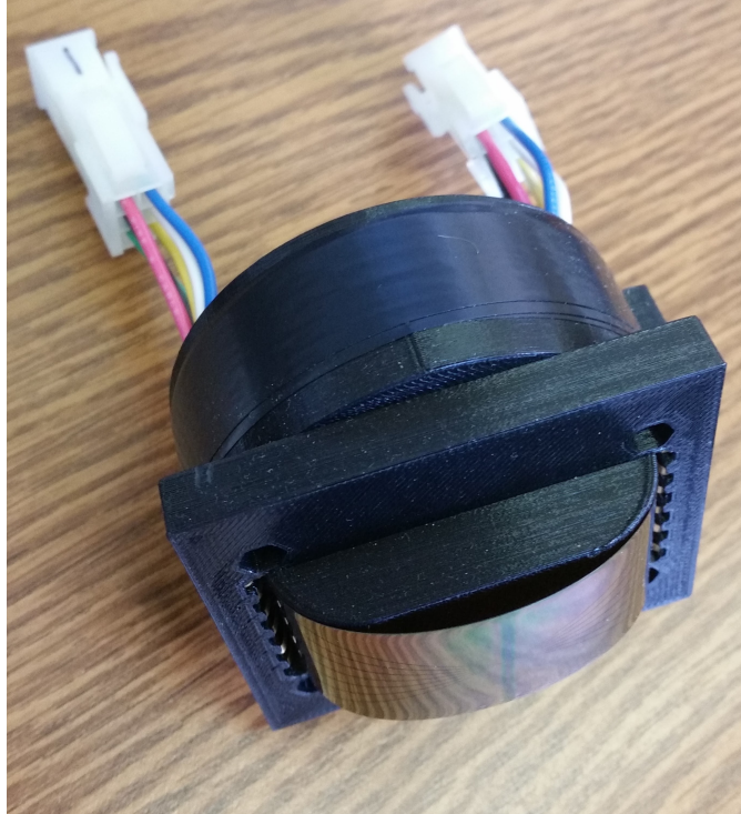
Figure 4.7: Custom 3D printed probe holder designed to house the \mu FPLP.
