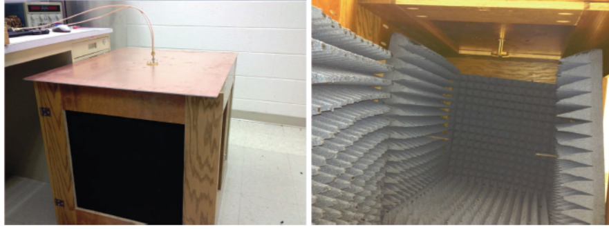
Figure 3.8: Photographs of S-parameter test in an anechoic chamber.
