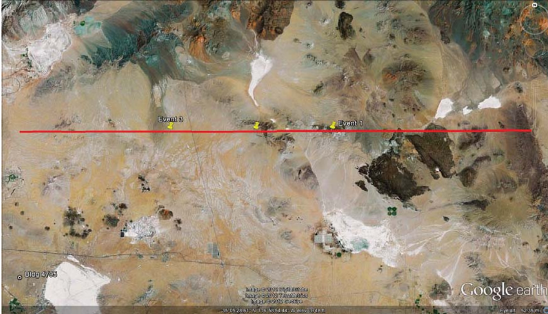
Figure 2.11: The 3 multipath events (reflection points) for the Black Mountain East-to-West run at EAFB using 5124 MHz.
