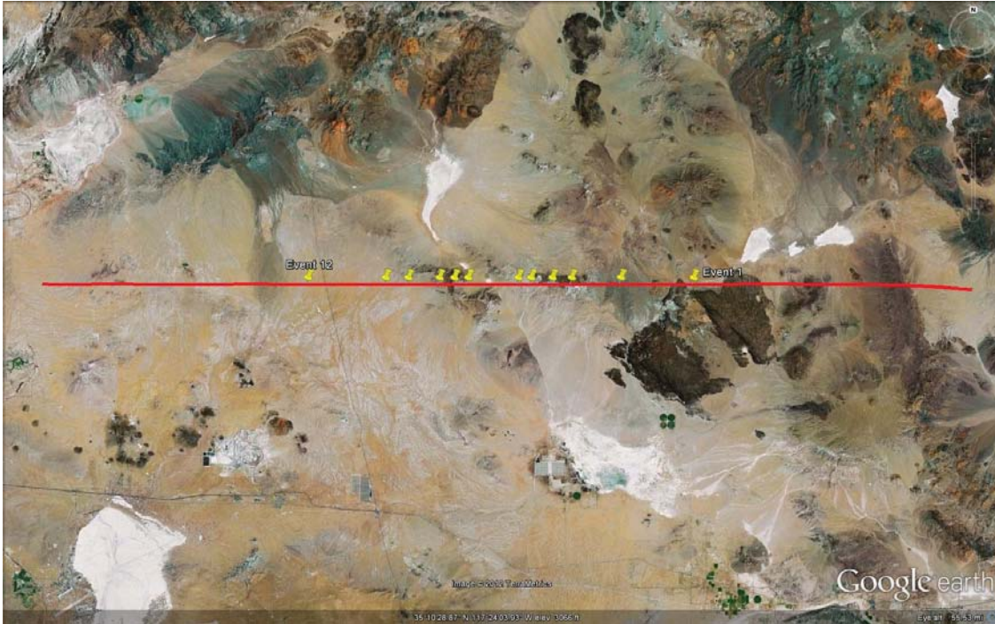
Figure 2.10: The 12 multipath events (reflection points) for the Black Mountain East-to-West run at EAFB using 1824 MHz. The yellow “thumb tack” markers indicate the multipath event locations. Event 1 is the rightmost marker and Event 12 is the left-most marker.
