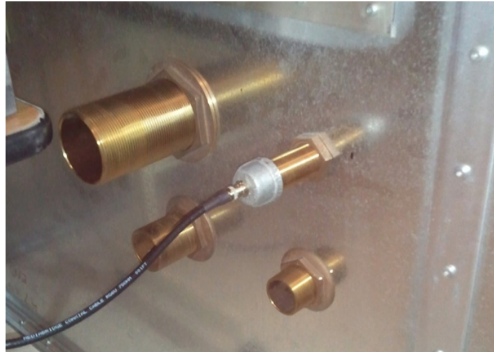
Figure 4-9. Inside view of the coupling connections on BYU's Faraday cage.
