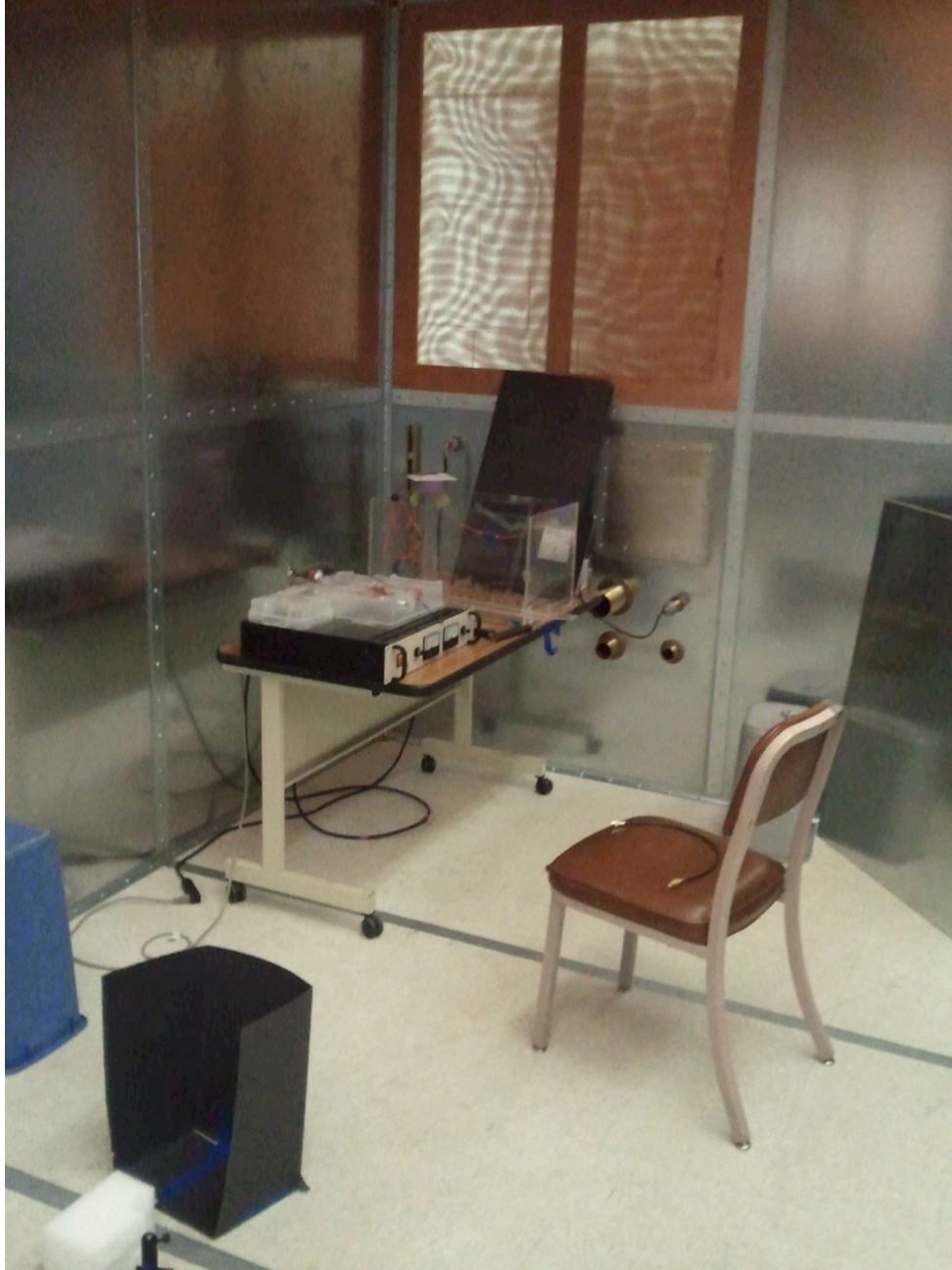
Figure 4-8. Inside view of the Faraday cage at BYU. A HV test setup such as this can be setup inside, and the double layered fine metallic mesh on the windows allows for natural light to reach the experimental setup but limits RF frequency penetration.
