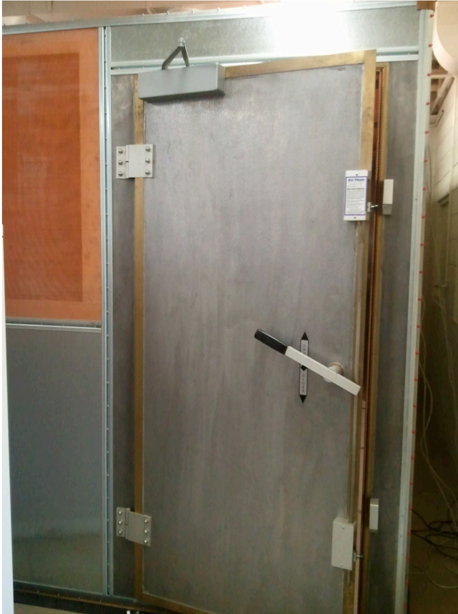
Figure 4-11. A metallic door offers access to the Faraday cage, but can be secured against RF penetration upon closure.
