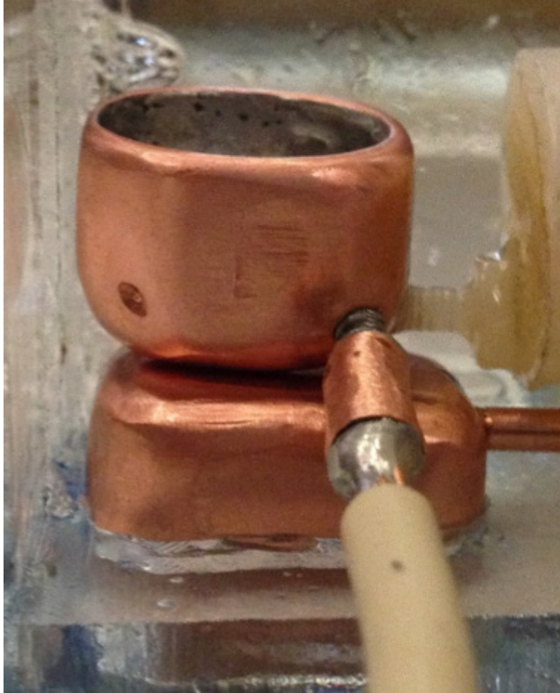
Figure 6-16. Surface contact for ‘down’ position for the switch shown in Figure 6-15. The flat base of the copper cup creates adequate contact with the bottom brass electrodes during the charging phase.
