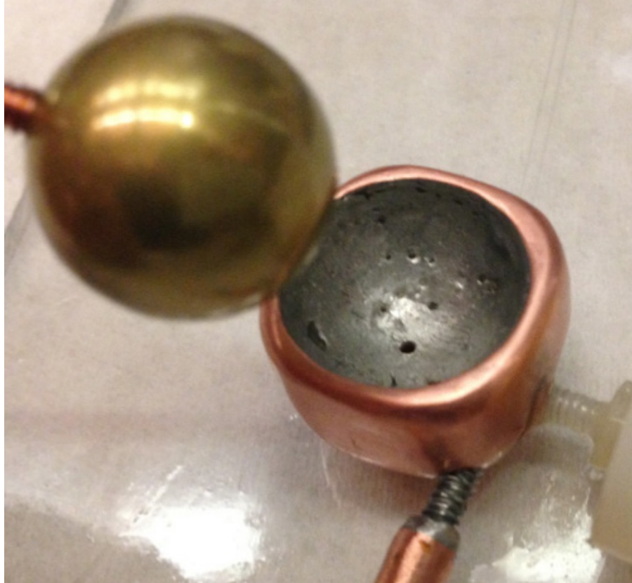
Figure 6-17. Surface contact for ‘up’ position for the switch shown in Figure 6-15. The molded solder-filled copper “cup” ensured optimum contact with the brass ball during the discharge phase.
