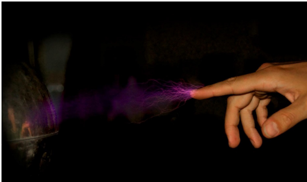
Figure 4-1. Corona discharge appearing as a purplish glow from the electric field produced between a charged Van de Graaff generator and a hand. Spindles of lightning protrude from the finger, showing the ionized conductive air pathways between the generator and the finger.
