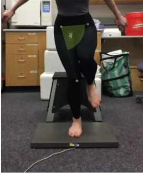
**Figure 3.** Participants landed on one foot from a height of 40 cm onto a portable force plate. The peak hip adduction angle was measured, using markers attached to the left ASIS, right ASIS, and patella of the landing leg.
