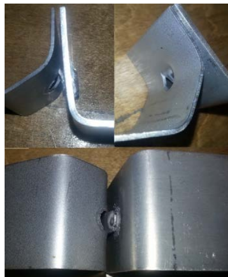
Figure 4-10 Nugget Joint Failure Large Steel Tear
