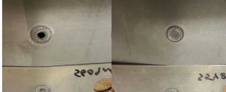
Figure 4-18 Cross-Tension with Nugget and Interfacial Failures
