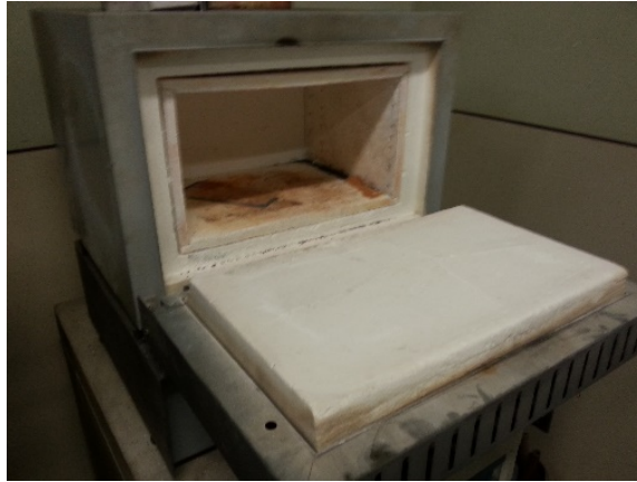
Figure 3-7 Oven for Warming Aluminum Coupon Before Bending
