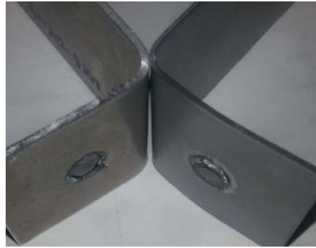
Figure 4-15 Interfacial Joint Failure
