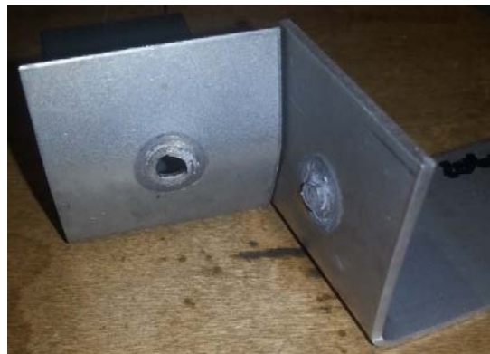
Figure 4-9 Nugget Joint Failure Small Steel Tear
