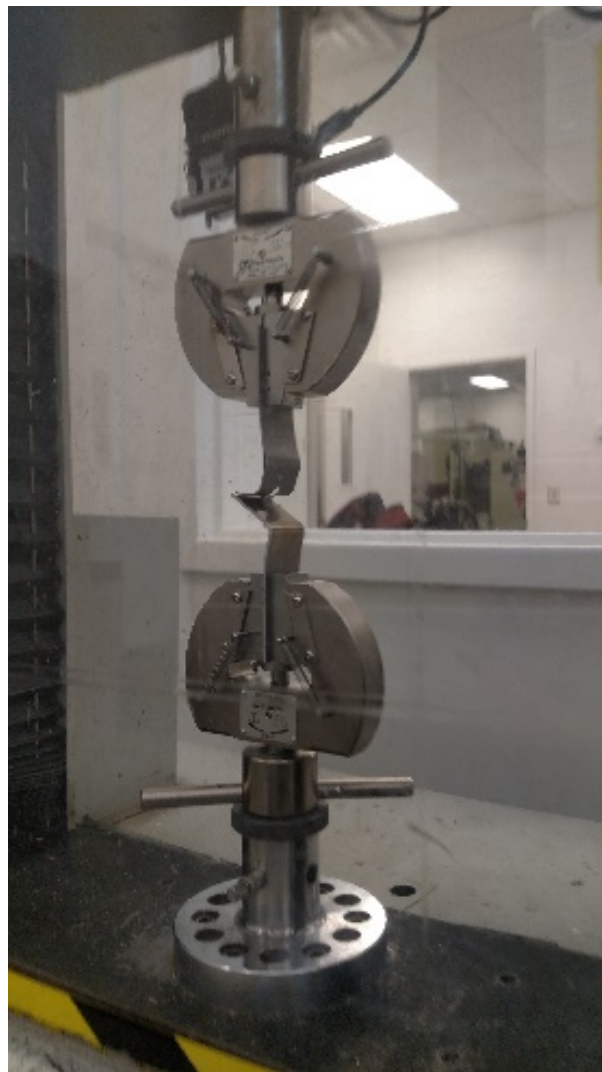
Figure 3-10 T-Peel Test as the Weld is Failing.
