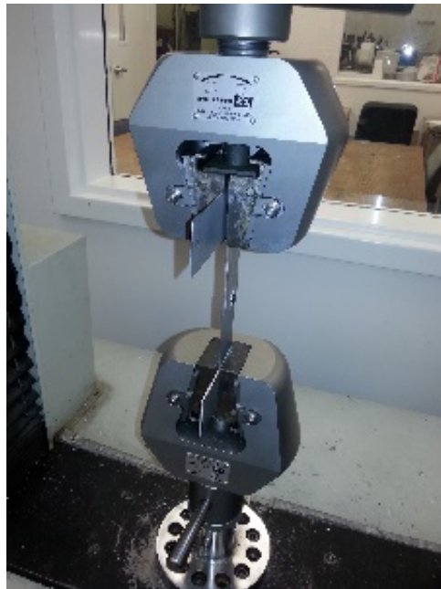
Figure 3-13 Shims to Align Coupons for Tension Testing
