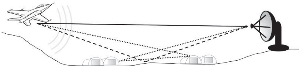
Figure 1.1: Multipath propagation in aeronautical telemetry. The solid line is the line-of-sight signal while the dashed lines are different propagation paths.
