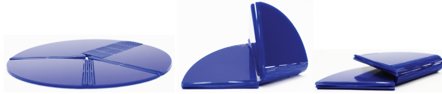
Figure 2.20: The strained joint technique applied to a degree 4 vertex.
