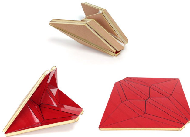
Figure 4.16: Prototype of split-vertex bird base thick origami mechanism fabricated from foam board and red polypropylene tape, demonstrating a flat surface with no holes.
