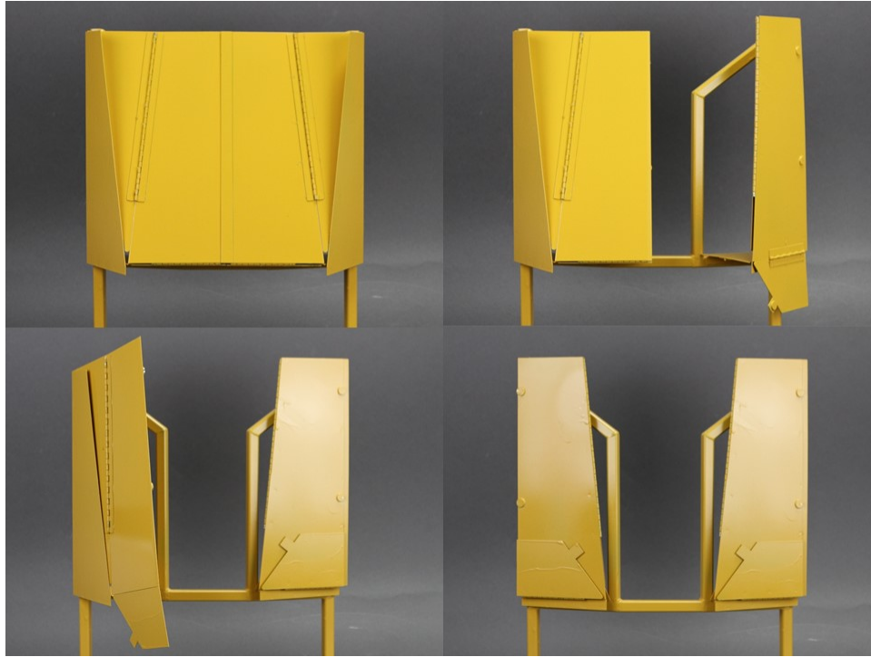
Figure 6.15: Eighth-scale prototype constructed from sheet metal.
