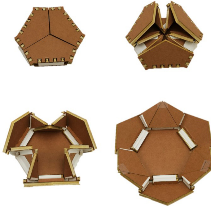
Figure 5.4: An under-developed hexagon pattern modified using the offset-panel technique.
