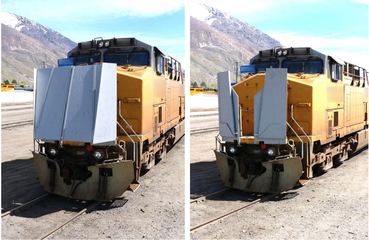
Figure 6.17: Full-scale prototype on a freight locomotive shown in both the stowed configuration (left) and deployed configuration (right). Photo has been modified to remove locomotive identity.
