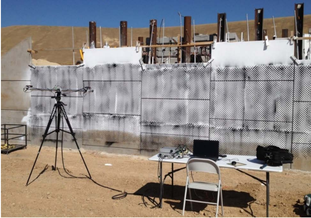
Figure 4-4. DIC setup in front of the MSE wall.
