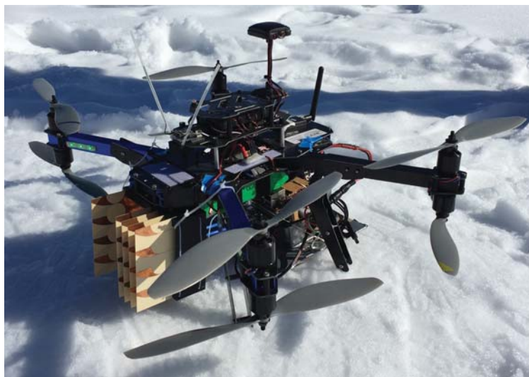
Figure 6.7: A picture of a X8 Octorotor with the radar attached on the bottom.
