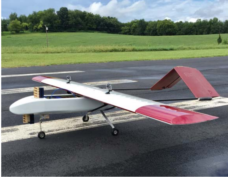
Figure 6.3: The BYU radar attached to VT's eSPAARO. The receiver and transmitter can be seen on the top and bottom of the front end of the fuselage.
