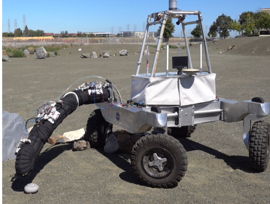
Figure 3.1: K-REX is a planetary rover developed by NASA for exploration in areas of rough terrain.
