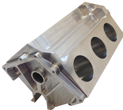
Figure 6.2: Engine block machined using tool paths generated by MUCAM team
