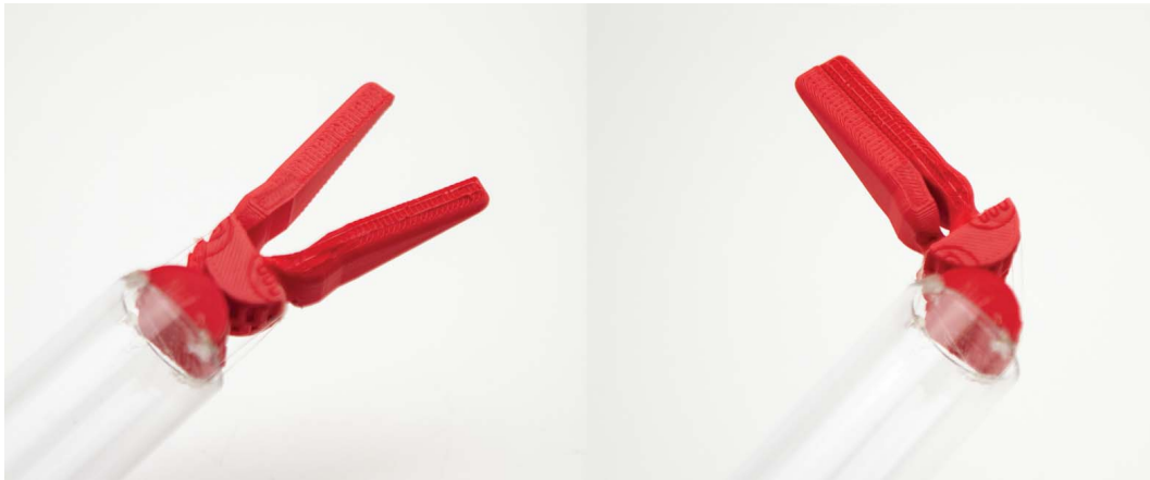
Figure 3.1: A 10:1 scaled prototype demonstrating two degrees of freedom.
