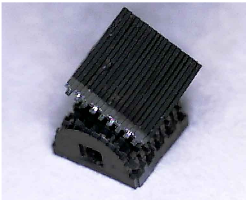
Figure 6.11: Micrograph of the assembled Crossed Cylinder Wrist with a more coarse stacking assembly ( 110\ \mu\text{m} layer thickness). The upper piece is rotated slightly about the axis of the lower and rolled slightly forward to demonstrate both directions of motion.
