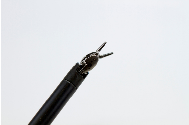
Figure 5.1: A surgical tool from Intuitive Surgical, Inc. mounted on a 2-DOF wrist. The tools shaft is approximately 8 mm in diameter.
