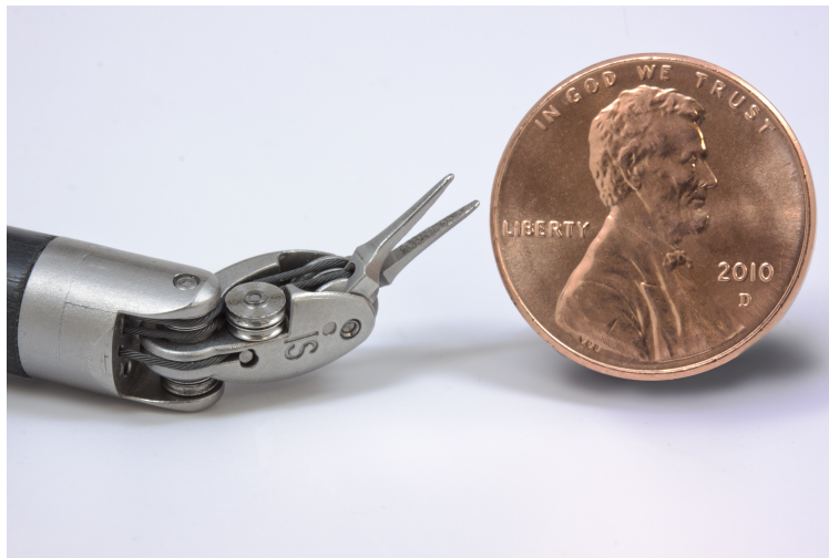
Figure 1.1: 8 mm Endowrist ® design by Intuitive Surgical. Image courtesy of Intuitive Surgical, Inc.
