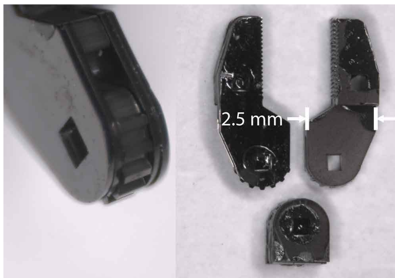
Figure 6.16: Photograph of the assembled geared portion of the Split CORE Grips (left) and a view of all the assembled elements (base piece and two grips) of the mechanism (right).
