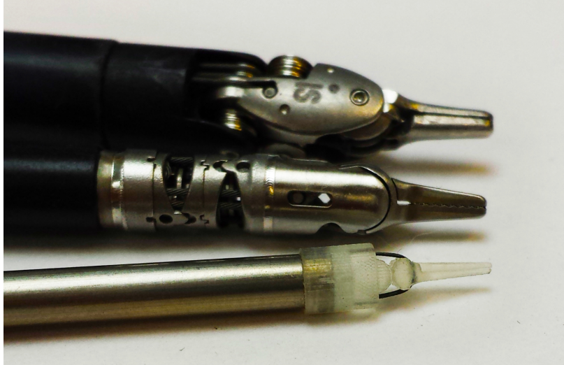
Figure 3.8: 3D printed Split CORE Grips attached to a 3.4 mm diameter instrument shaft. 5 and 8 mm diameter instruments shown for comparison.
