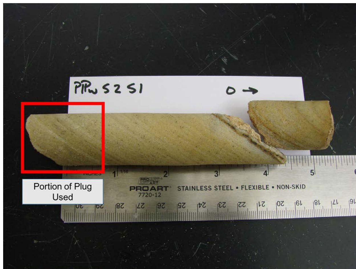
Figure 4. An example of a sample from the Weber S2 dune extracted using a 1-inch diameter core plug drill. Note that even with just a 1-inch diameter core, several different laminae were sampled. Whenever possible, the portion of the plug farthest from the exposed surface was used for XRF analysis to avoid surface effects. The approximate portion of this plug used is shown in the red box.
