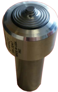
Figure 2-2: Q70 Friction Stir Processing Tool with 8 mm-long, Threaded Conical Pin and 25 mm Diameter Convex Shoulder.
