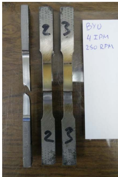
Figure 4-6: Tensile Failure of Z-Depth Control Specimen 4I-250R
