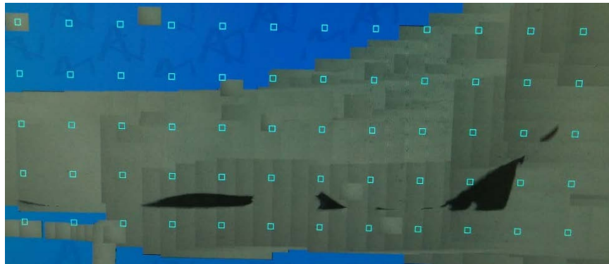
Figure 3-4: Micro-Hardness Testing: Indent Grid
