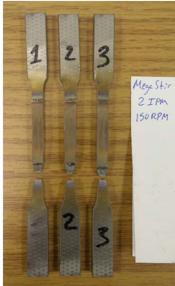
Figure 4-7: Tensile Failure of Z-Force Control Specimen 2I-150R
