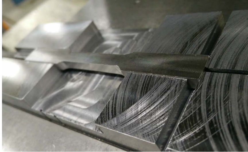
Figure 3-2: CNC-Machined Dogbone in Custom Fixture
