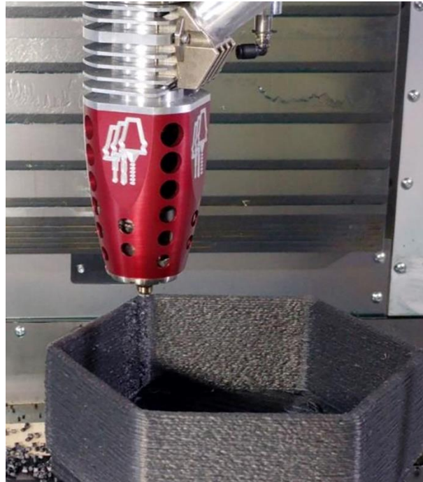
Figure 1. AMBIT XTRUDE FGF extruder mounted in a HAAS TM-2P CNC mill.
