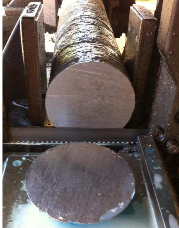
Figure 6. Ingot from melt run #1 after removing the dovetail
