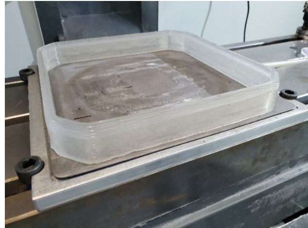
Figure 4. Recycled PETG print.
