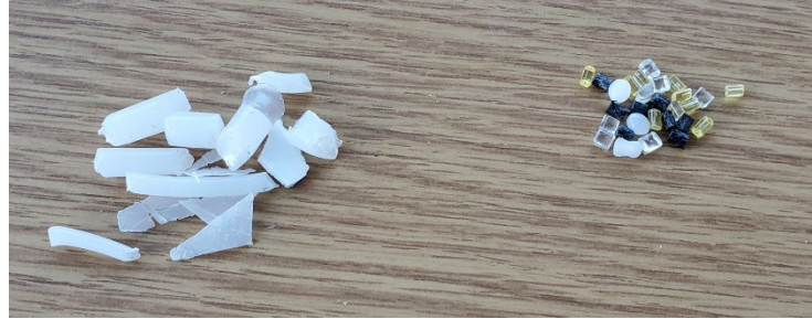
Figure 1. Recycled material after one granulator cycle (left) next to standardized pellets (right).
