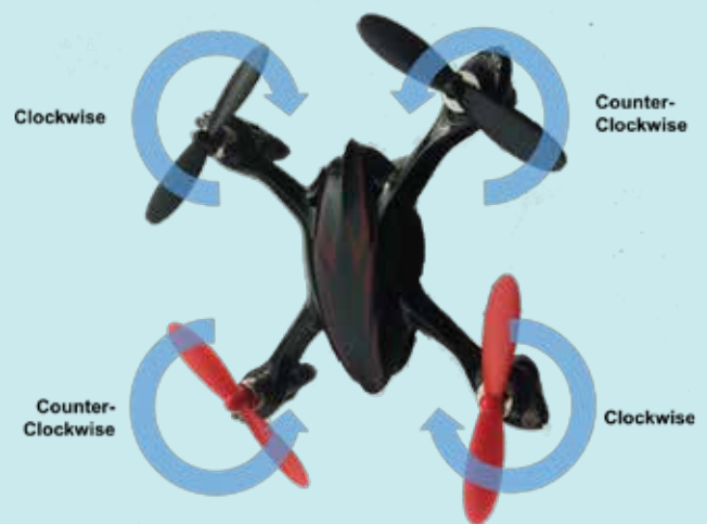
Figure 2. The spinning rotors of a quadcopter.
