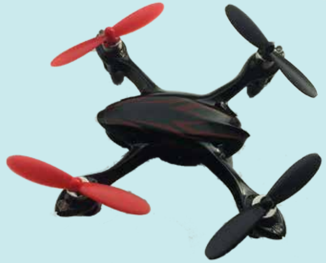
Figure 1. Quadcopters use four propellers to generate lift.
