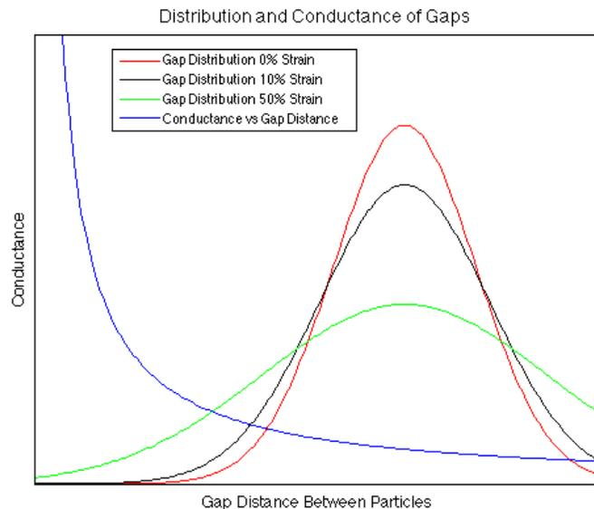
Figure 3.6 – Gap distances with strain and gap conductance
