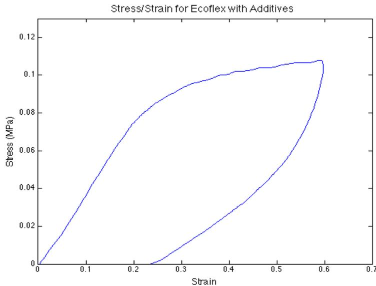
Figure 2.4 – Loading and unloading of an Ecoflex gauge with 5% NiNs and 1.5% NCCF
