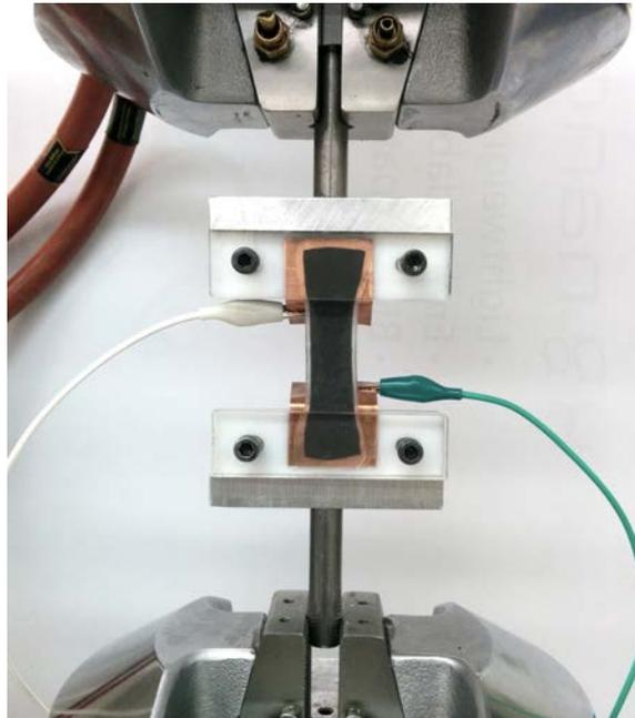
Figure 3.2 – Testing setup with insulating grips
