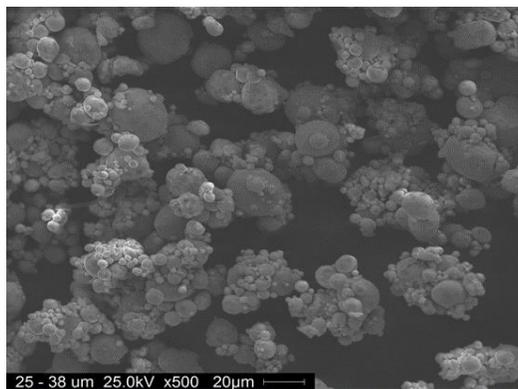
**Figure 1. Powder agglomerates cured at  $100^\circ\text{C}$  produced using the procedure above; at  $25\mu\text{m}$ - $38\mu\text{m}$**
