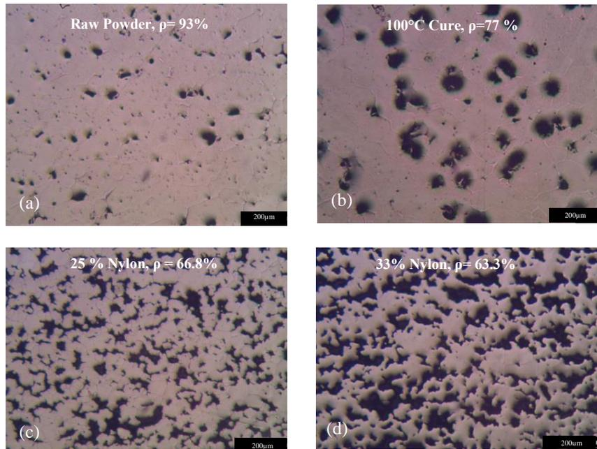
**Figure 4. The porosity on the cross-section of the samples made by feedstock materials:**
