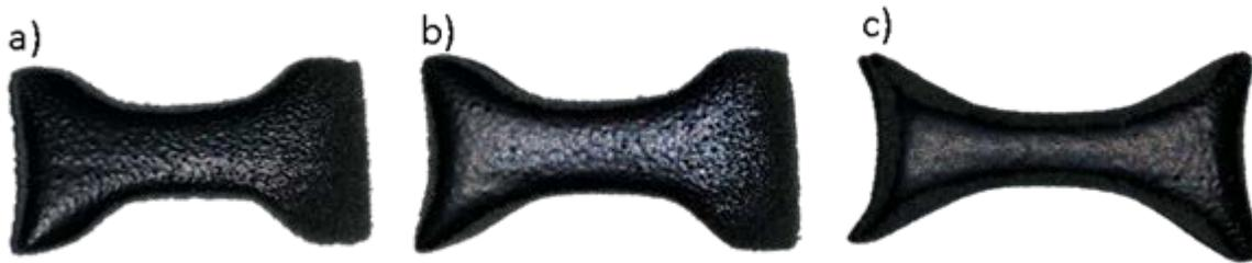
Figure 5 - Tensile specimens made with the same energy density ( $4.0 \text{ J/cm}^2$ ), a) 4.0s of exposure time with  $1.0 \text{ W/cm}^2$  power density, b) 3.33s of exposure time with  $1.2 \text{ W/cm}^2$  power density, c) 2.0s of exposure time with  $2.0 \text{ W/cm}^2$  power density. The degree of sintering is decreased as exposure time increases as evident by the rougher surface finish.
