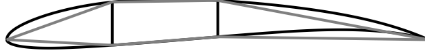
Figure 7: Airfoil section divided up into several flat buckling panels by the section's webs
