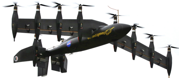
Fig. 2 NASA GL-10 eVTOL prototype aircraft during vertical takeoff. Credits: NASA Langley/David C. Bowman.
