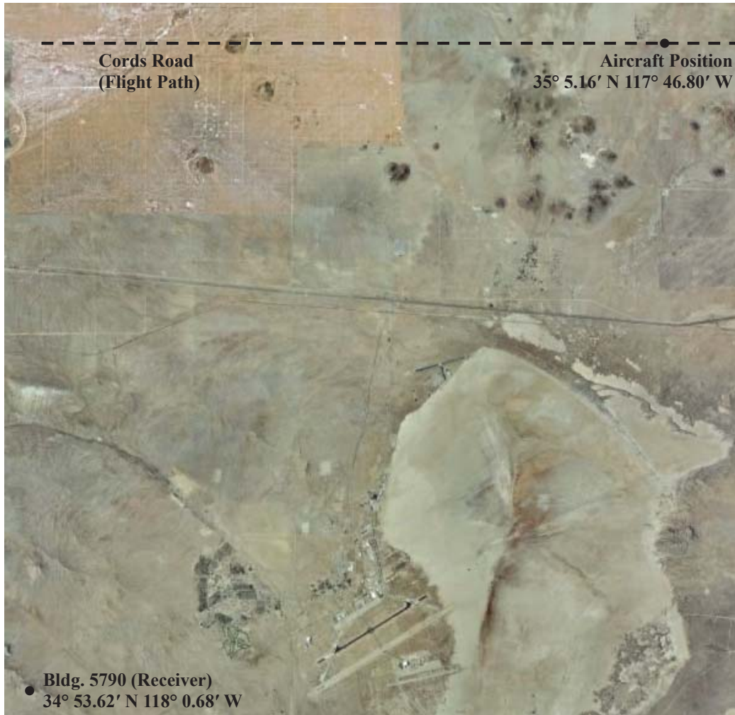
Figure 2.2: A map showing the positions used to define the 2-ray channel multipath channel scenario for Edwards AFB.
