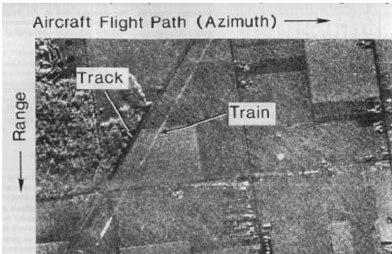
Figure 3.14: Actual SAR image of a train moving mostly in the cross-track direction, shifted off its tracks due to the cross-track component of its motion. (Source: [74])
